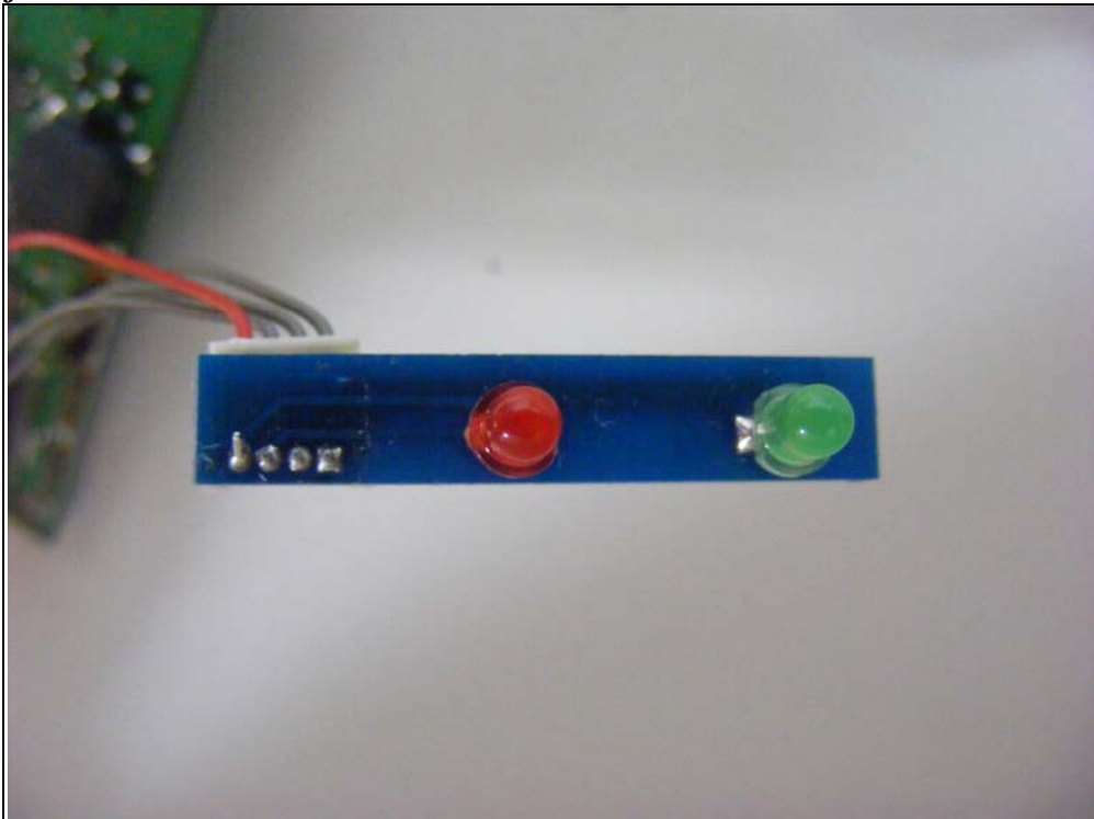
Bottom view of LED PCB
