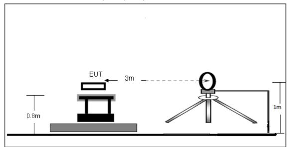
(B) Radiated Emission Test-Up Frequency 30MHz~1GHz
