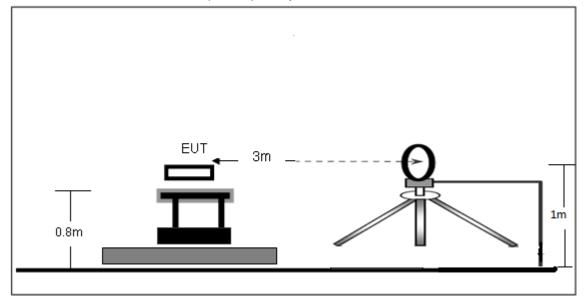
(B) Radiated Emission Test-Up Frequency 30MHz~1GHz
