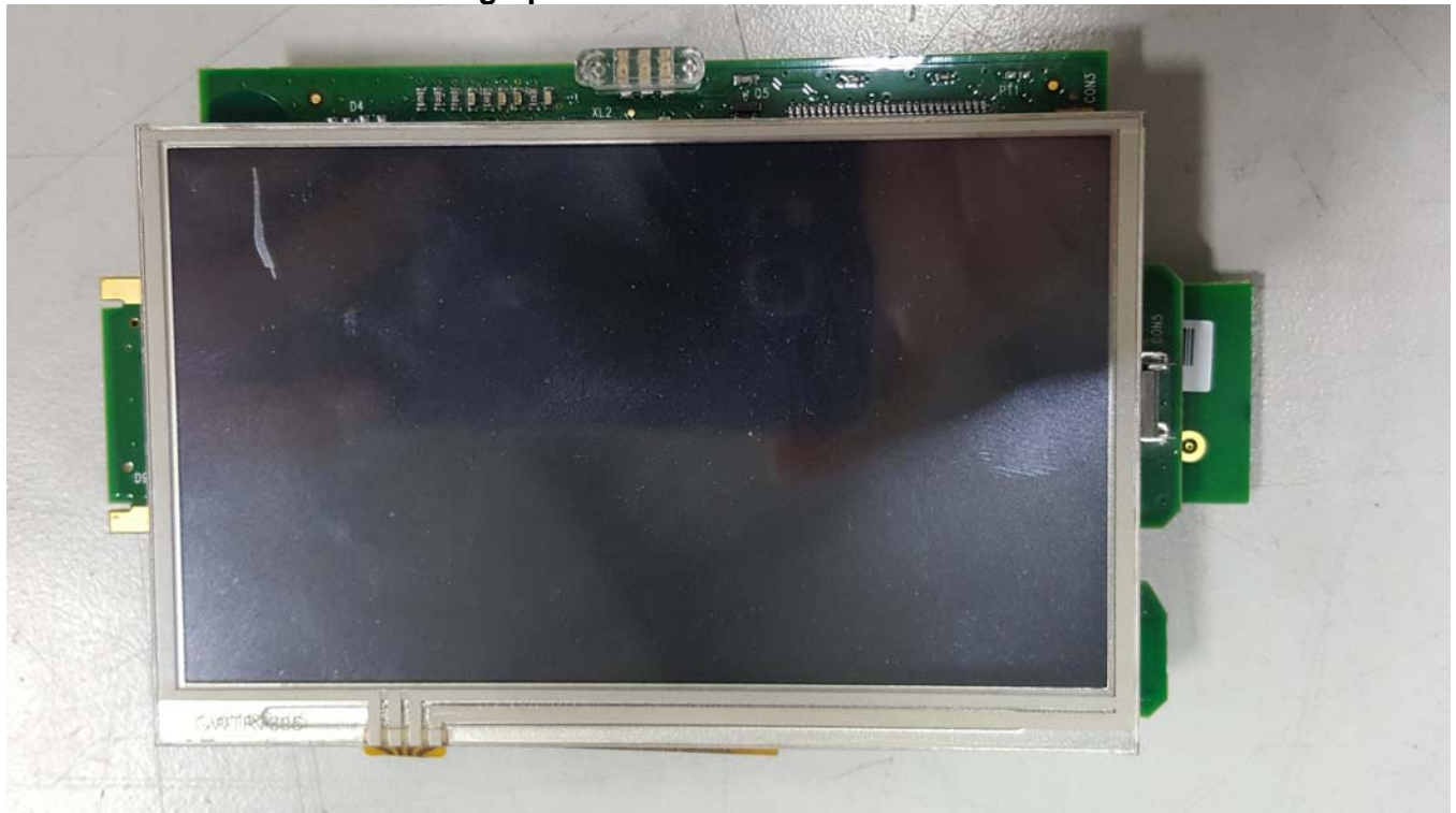
Photograph of Main Board with LCD installed
