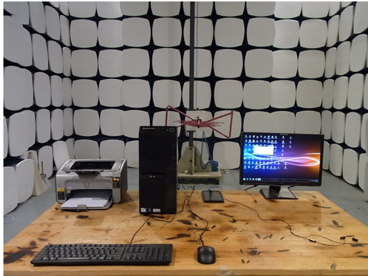
Radiated Emission above 1GHz
