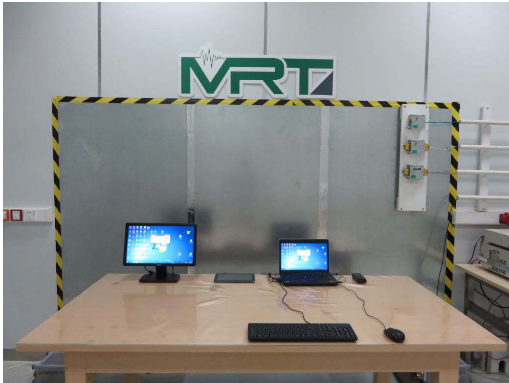
Description: Back View of the Conducted Emission Test Setup
