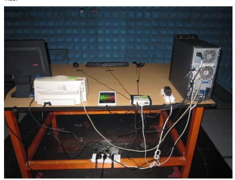
FCC Part15B Radiated Emission above 1GHz Setup 1- EUT+ Battery +PC+ LCD monitor -Front
