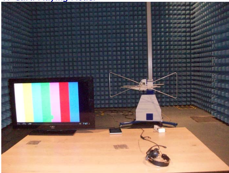
Radiated Emission Test Set-up -below 1GHz
