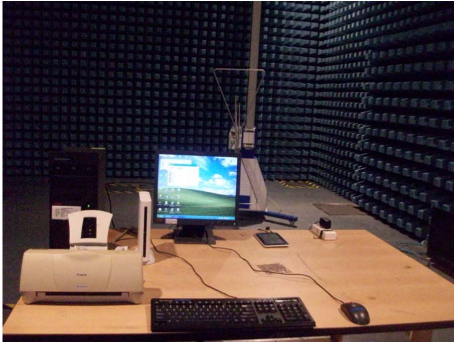
Radiated Emission Test Set-up-Below 1GHz
