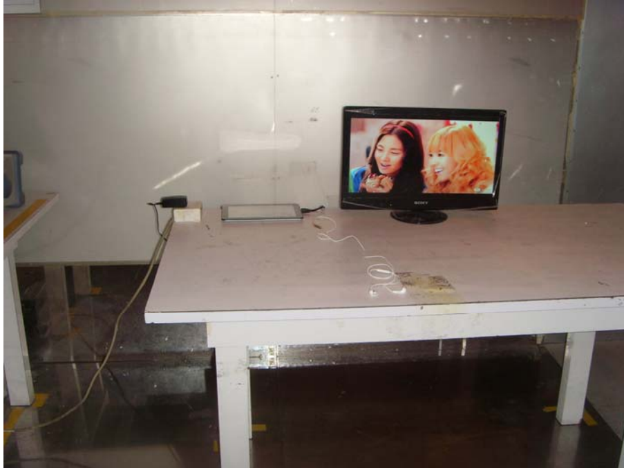
Conducted Emission Test Set-up (TF Card playing mode)
