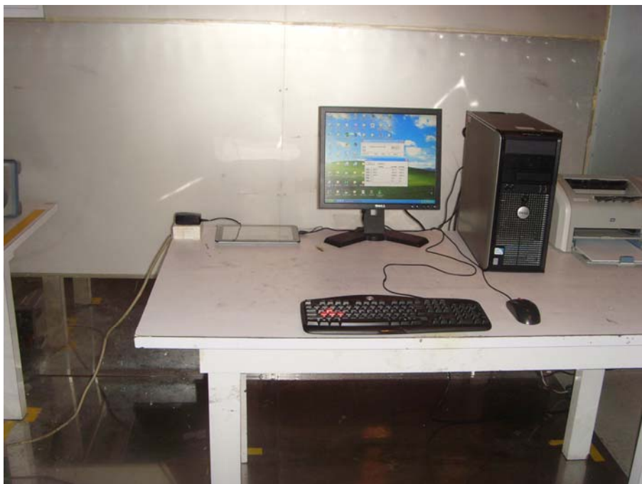
Conducted Emission Test Set-up (Connected to PC mode)
