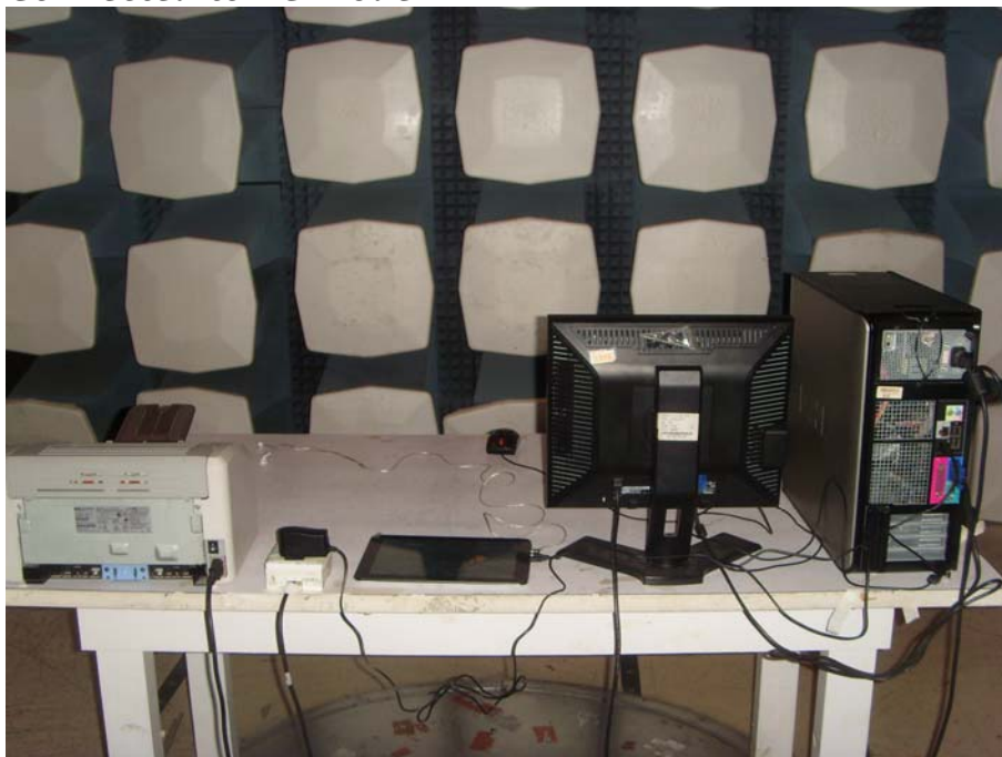
Radiated Emission Test Set-up (Rear view)
