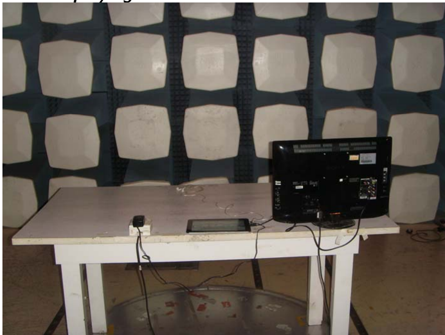
Radiated Emission Test Set-up (Rear view)
