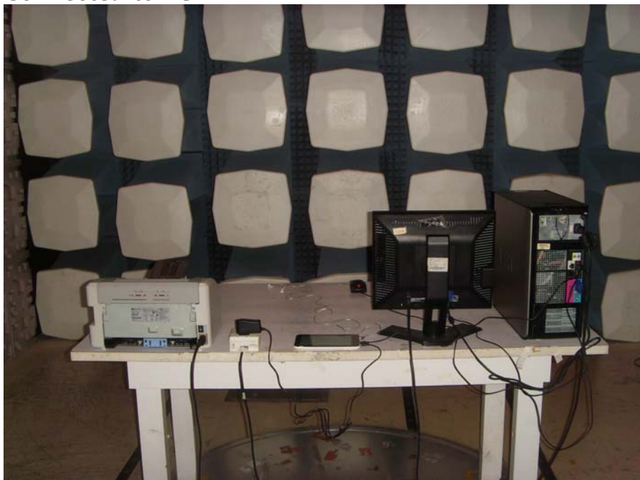
Radiated Emission Test Set-up (Rear view)
