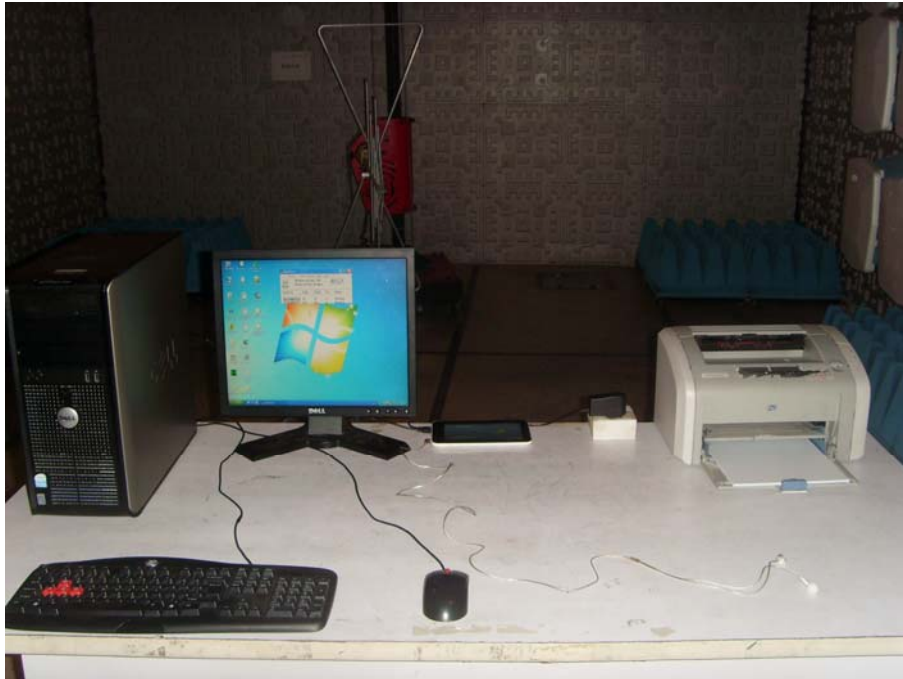
Radiated Emission Test Set-up (Front View)
