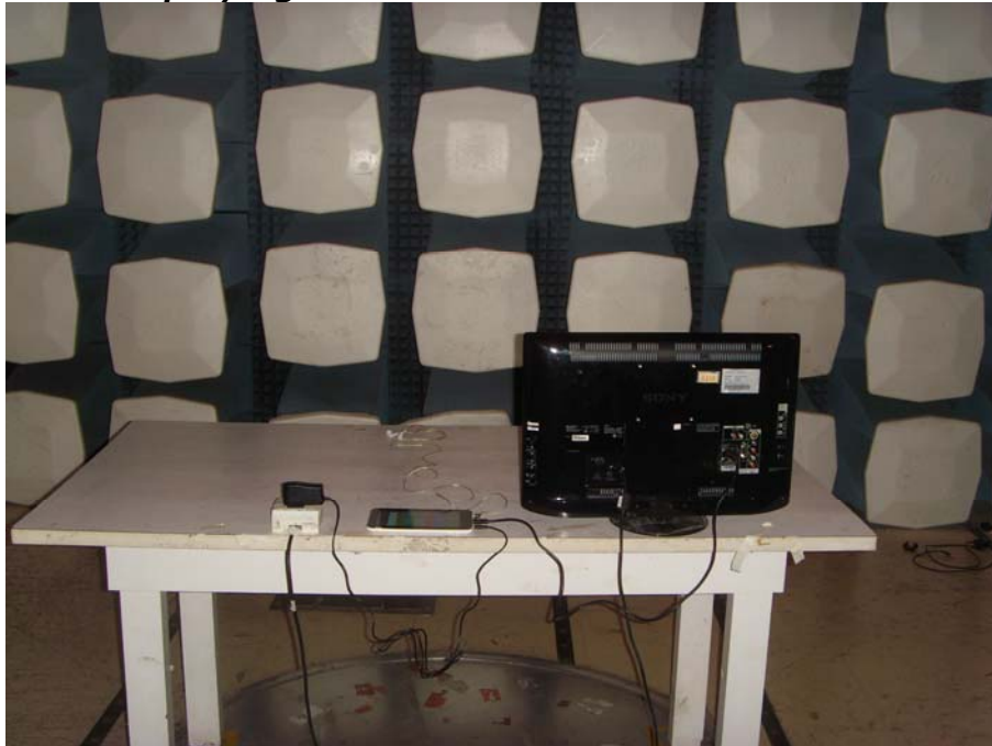
Radiated Emission Test Set-up(Rear View)
