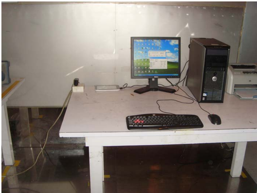
Conducted Emission Test Set-up(Connected to PC mode)
