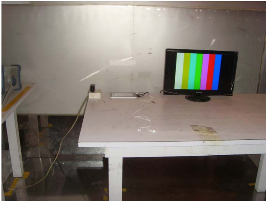
Conducted Emission Test Set-up(TF Card Playing Mode)
