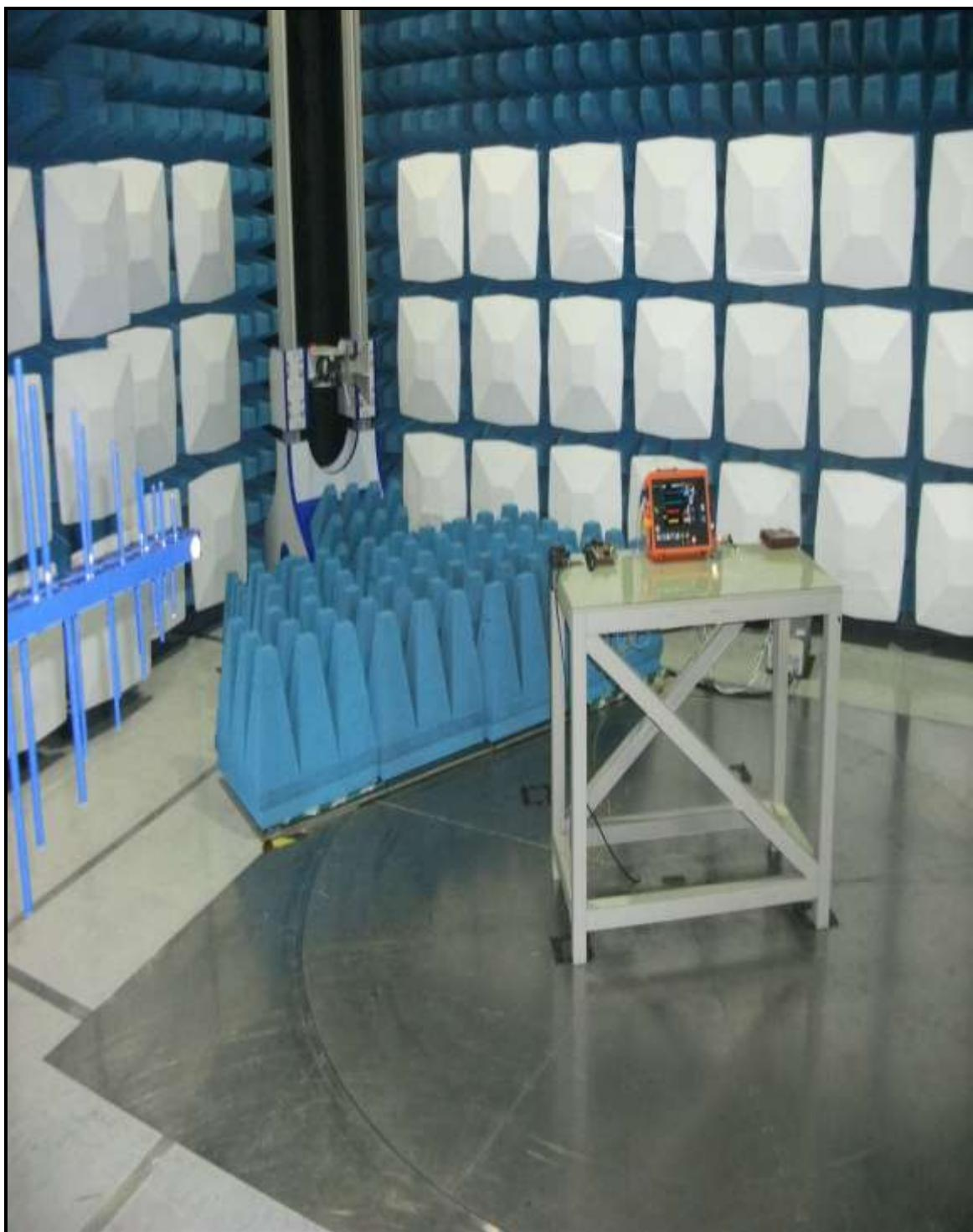
**PHT\87862JD01\005 - Test Configuration Photograph - FCC Radiated 002**
