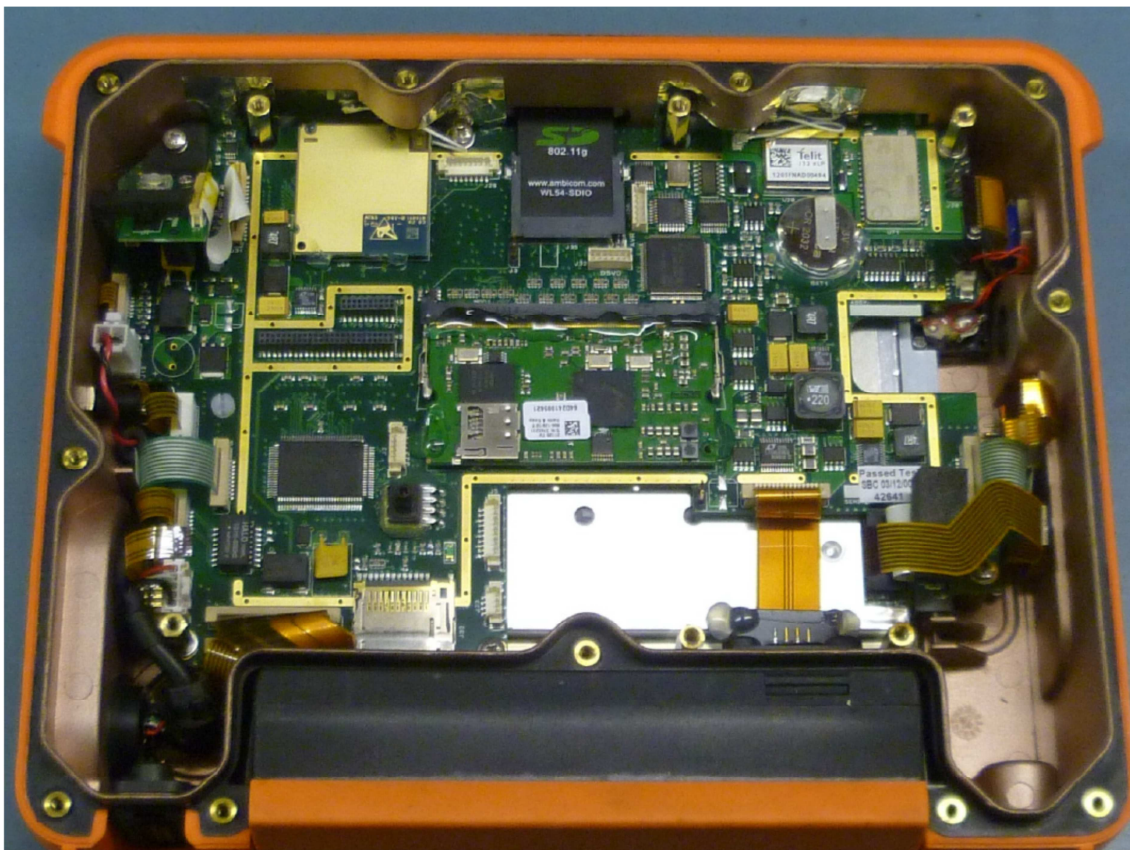
TempusIC host internal view 2 (showing radio module positions)
