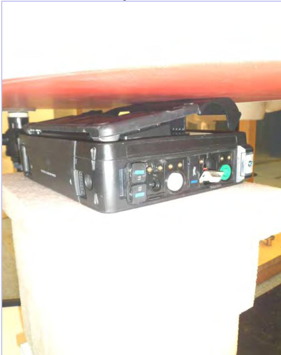
**Note:** EUT was configured with the most conservative and the RF antenna is at closest separation distance to the phantom flat section.
