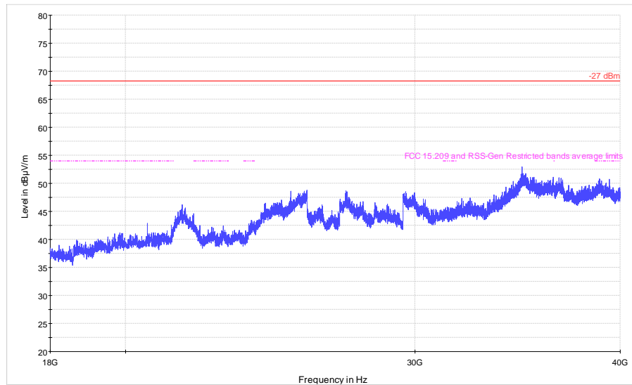
Figure 8.8-41: Cabinet spurious emissions 18 - 40 GHz, 10 MHz Channel
