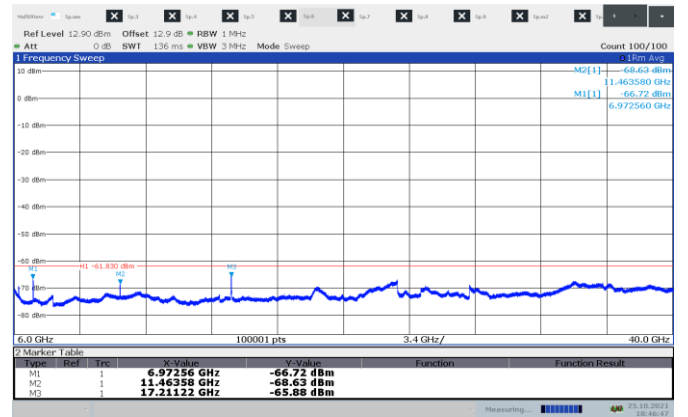
Figure 8.8-20: Conducted peak spurious emissions 1- 40 GHz on low channel 20 MHz sample plot
