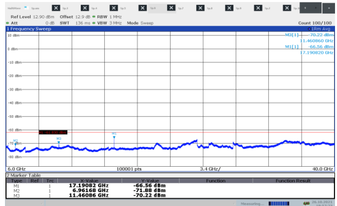
Figure 8.8-2: Conducted peak spurious emissions 1- 40 GHz on low channel 10 MHz sample plot
