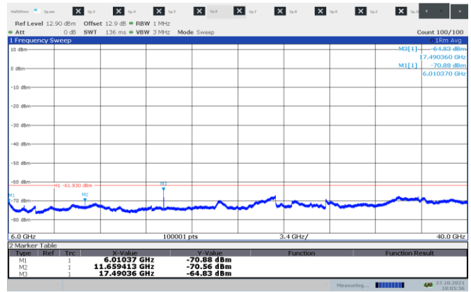
Figure 8.8-16: Conducted peak spurious emissions 1-40 GHz on 5830 MHz channel 10 MHz sample plot
