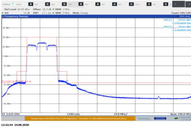
Figure 8.4-7: Emission measurement outside 10 MHz from the SAS assigned channel edge, sample plot for 10 MHz 3cc low channel
