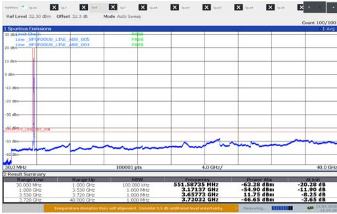
Figure 8.5-16: : Conducted spurious emissions for 20 MHz 3cc low channel sample plot 30 MHz – 40 GHz
