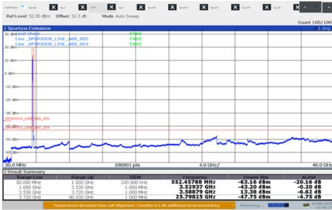
Figure 8.5-11: Conducted spurious emissions for 20 MHz 2cc low channel sample plot 30 MHz – 40 GHz
