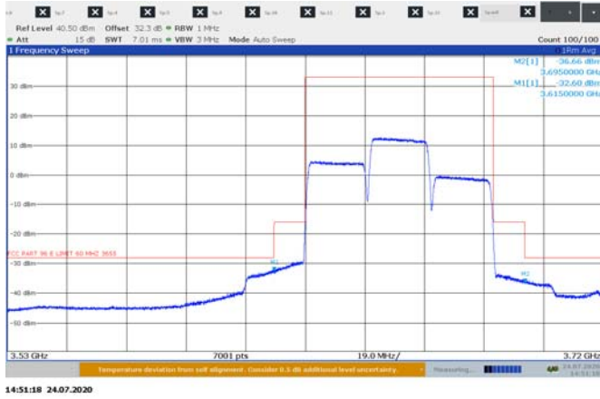
Figure 8.4-25: Emission measurement outside 10 MHz from the SAS assigned channel edge, sample plot for 20 MHz 3cc additional high channel
