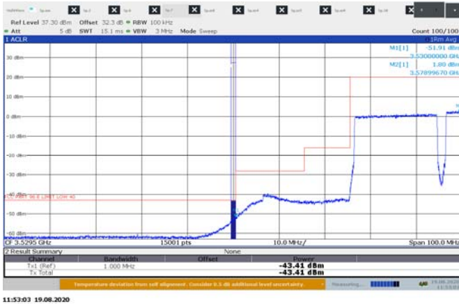
Figure 8.5-14: Low Bandedge for 20 MHz 2cc channel at 3530 MHz sample plot
