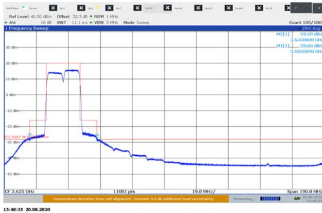
Figure 8.4-1: Emission measurement outside 10 MHz from the SAS assigned channel edge, sample plot for 10 MHz 2cc low channel
