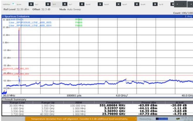
Figure 8.5-1: : Conducted spurious emissions for 10 MHz 2cc low channel sample plot 30 MHz – 40 GHz
