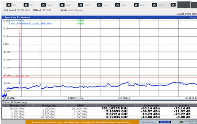
Figure 8.5-6: : Conducted spurious emissions for 10 MHz 3cc low channel sample plot 30 MHz – 40 GHz
