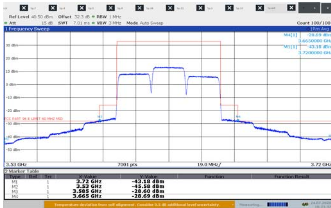
Figure 8.4-19: Emission measurement outside 10 MHz from the SAS assigned channel edge, sample plot for 20 MHz 3cc low channel
