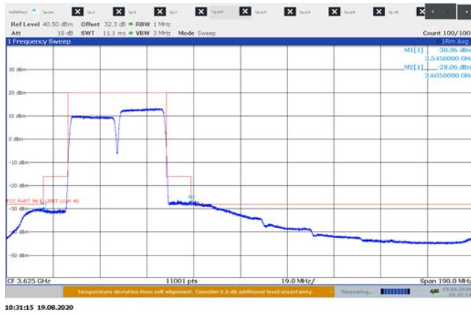
Figure 8.4-13: Emission measurement outside 10 MHz from the SAS assigned channel edge, sample plot for 20 MHz 2cc low channel
