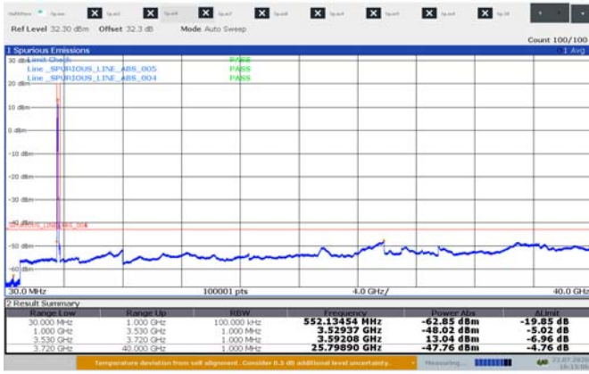
Figure 8.5-16: : Conducted spurious emissions for 20 MHz 3cc low channel sample plot 30 MHz – 40 GHz
