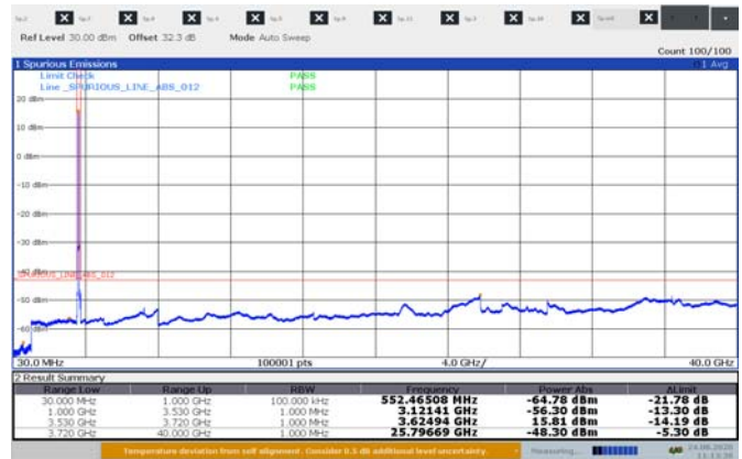
Figure 8.5-7: : Conducted spurious emissions for 10 MHz 3cc mid channel sample plot 30 MHz – 40 GHz
