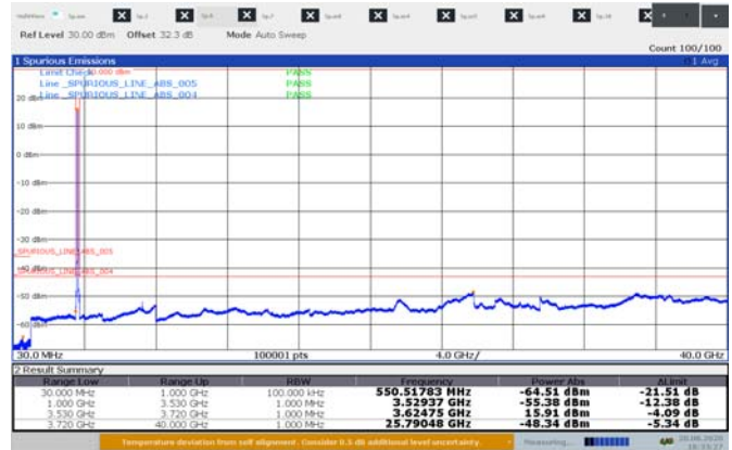
Figure 8.5-2: : Conducted spurious emissions for 10 MHz 2cc mid channel sample plot 30 MHz – 40 GHz
