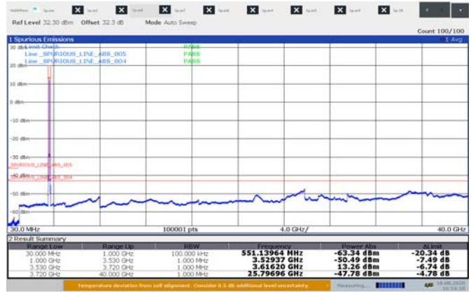
Figure 8.5-12: Conducted spurious emissions for 20 MHz 2cc mid channel sample plot 30 MHz – 40 GHz
