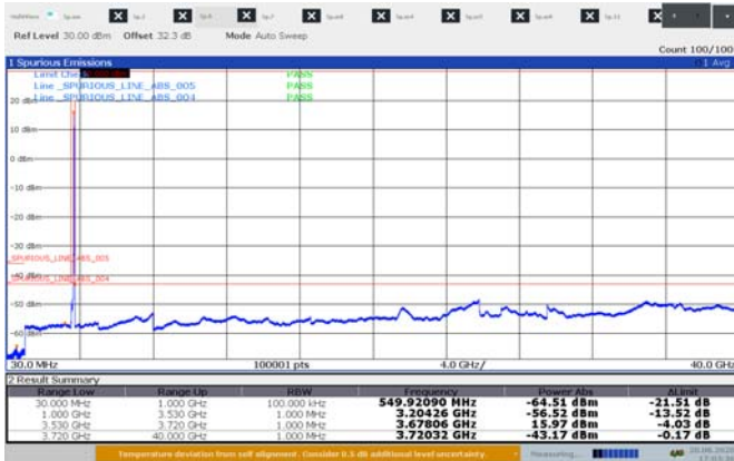
Figure 8.5-1: : Conducted spurious emissions for 10 MHz 2cc low channel sample plot 30 MHz – 40 GHz
