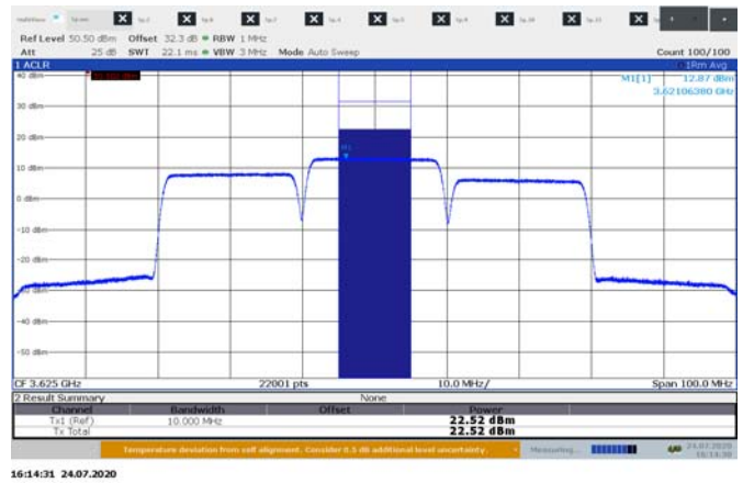
Figure 8.1-8: : Ouput power dBm/10 MHz sample plot, 3cc, 20 MHz channel
