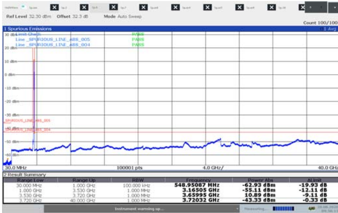
Figure 8.5-11: Conducted spurious emissions for 20 MHz 2cc low channel sample plot 30 MHz – 40 GHz
