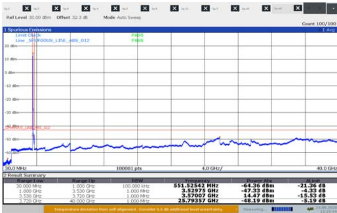
Figure 8.5-6: : Conducted spurious emissions for 10 MHz 3cc low channel sample plot 30 MHz – 40 GHz
