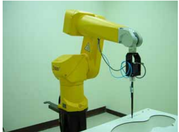
Fig. 5.2 Probe setup on robot
