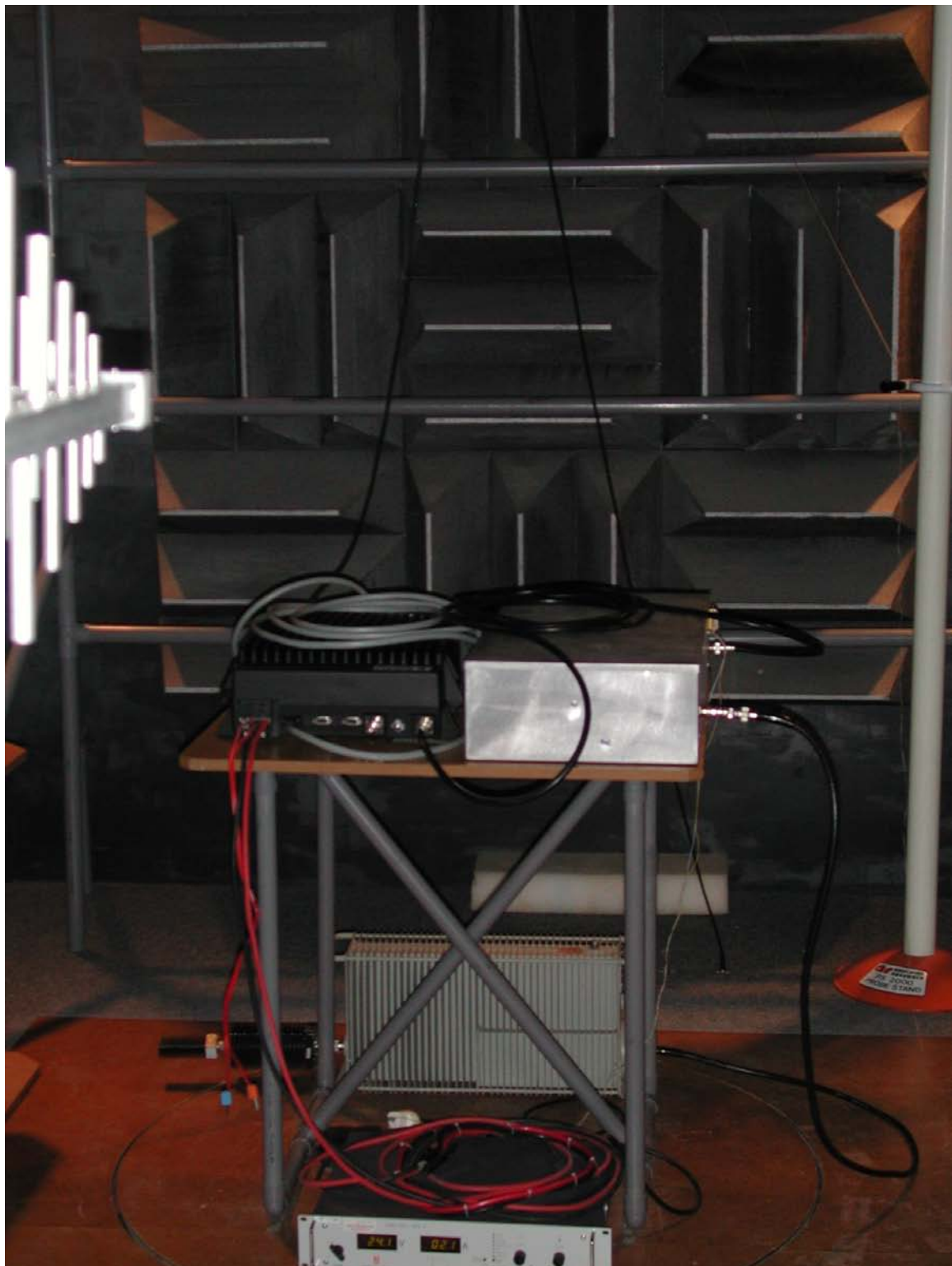
Photograph 1: Test setup cabinet radiation (> 30 MHz); view 1
