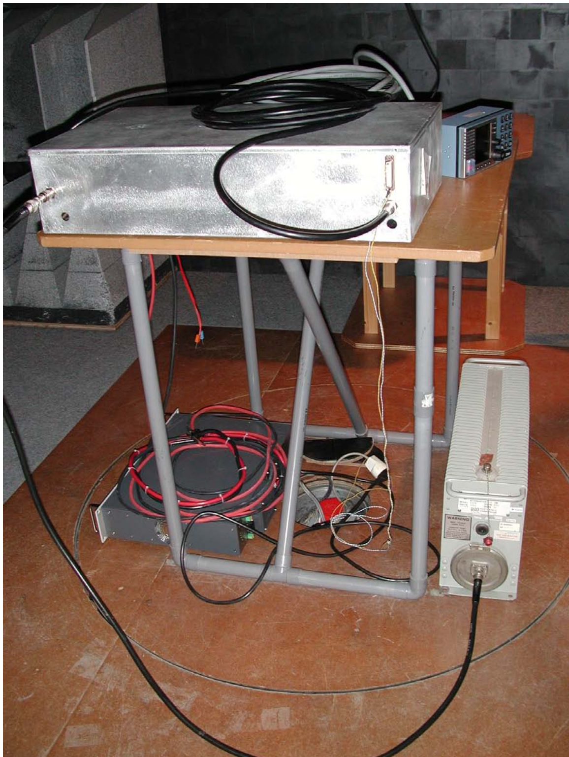
Photograph 2: Test setup cabinet radiation (> 30 MHz); view 2
