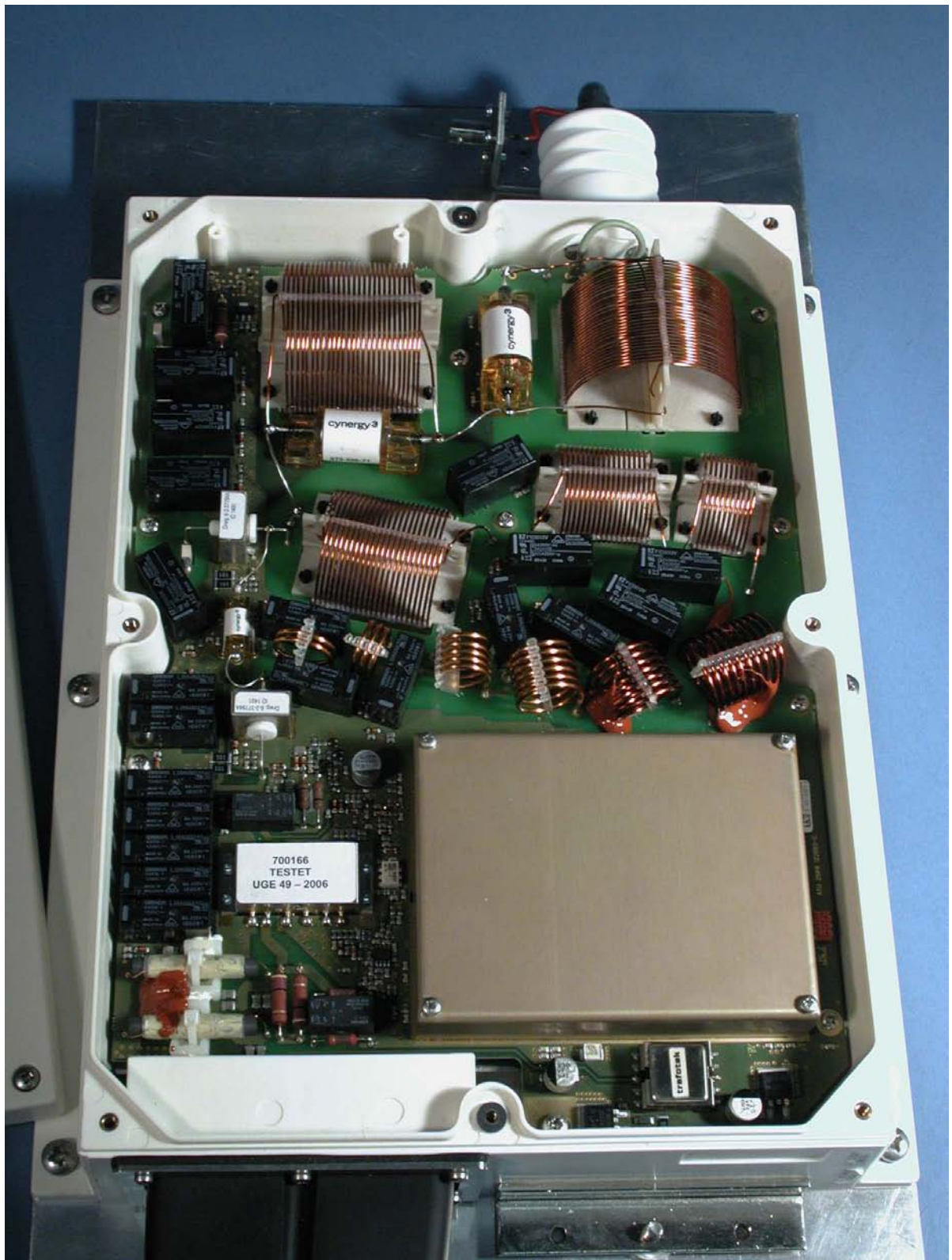
Photograph 8: Antenna tuner unit SAILOR ATU5215 internal view
