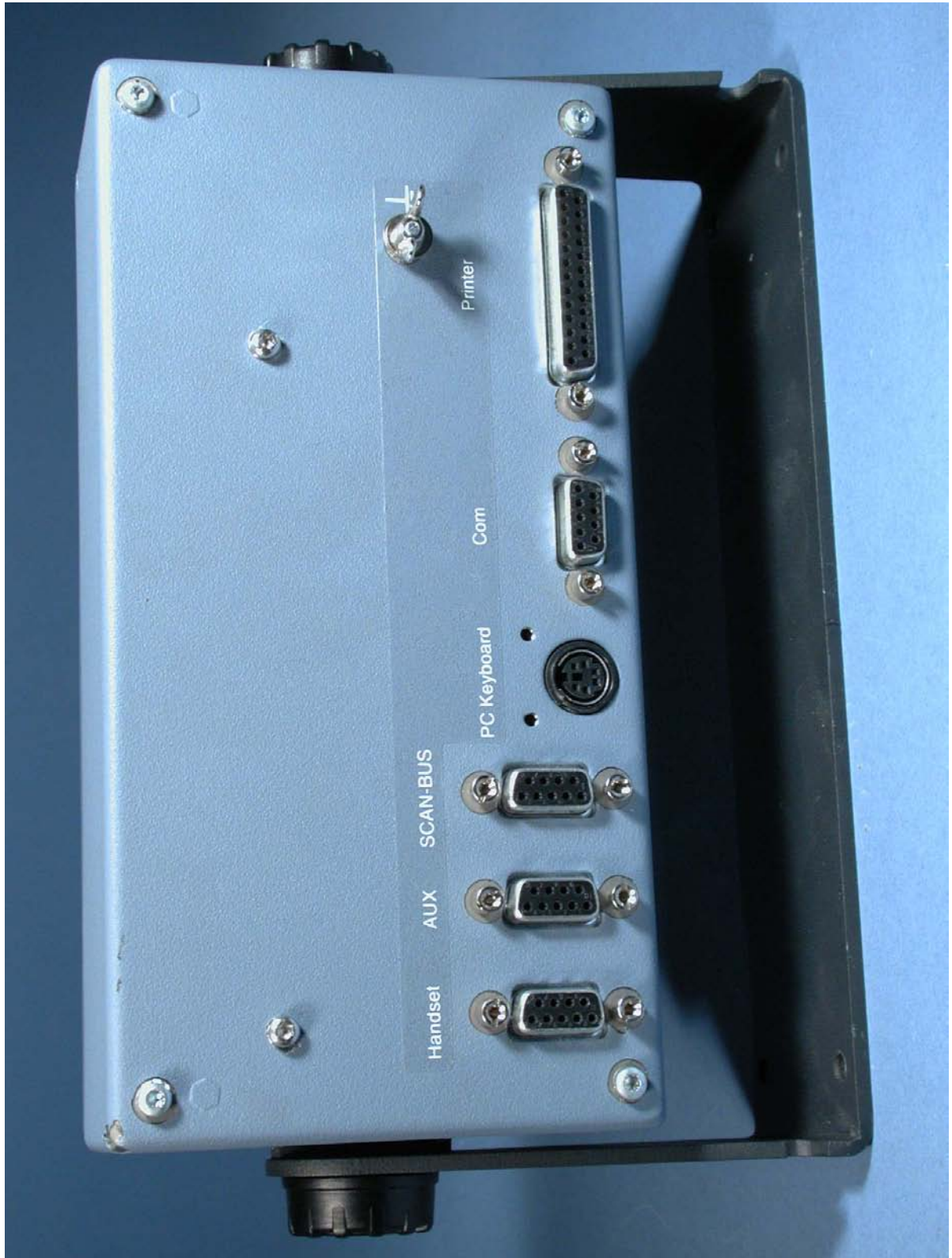
Photograph 4: Control unit CU5100 rear view
