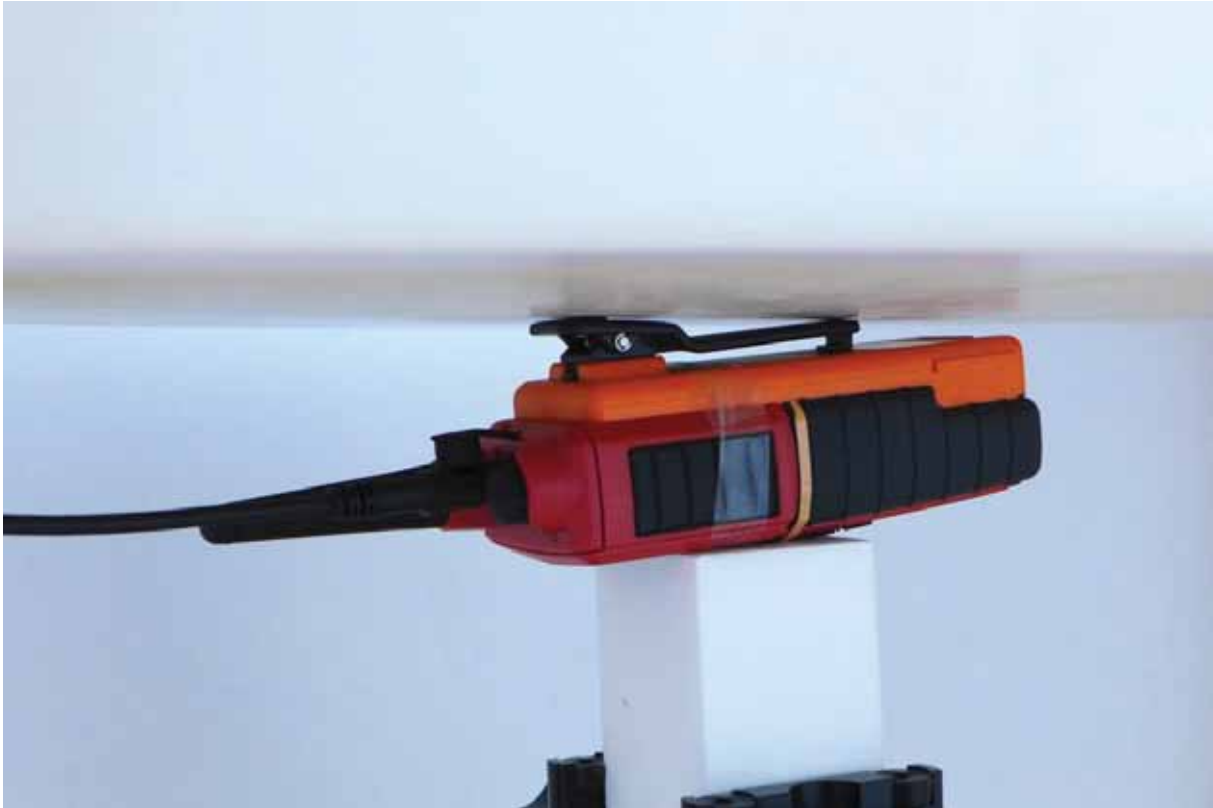
Pic. 6: Test position back side of EUT towards the phantom, belt clip and PTT microphone (C500) attached, 0 mm distance.
