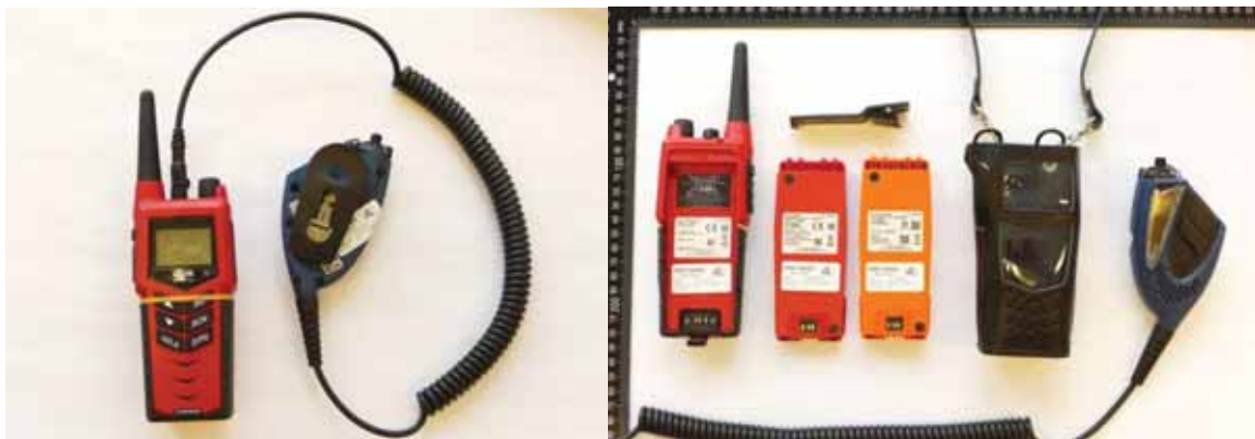
Pic. 3: Device under test with attached PTT microphone and tested accessory (B3906, B3503, belt clip, leather case, C500).
