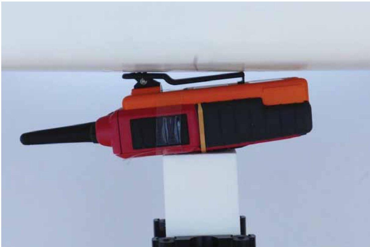
Pic. 5: Test position back side of EUT towards the phantom, belt clip attached, 0 mm distance.
