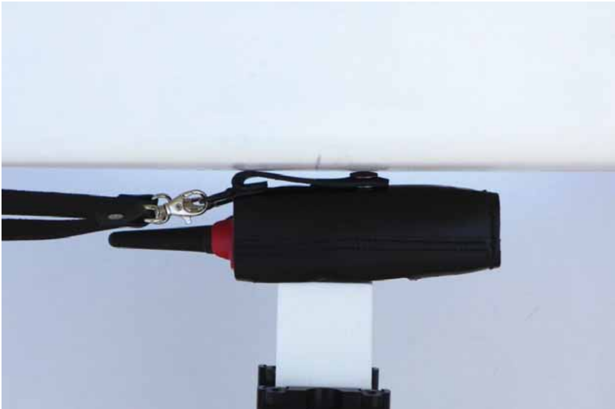
Pic. 7: Test position back side of EUT towards the phantom, leather case attached, 0 mm distance.
