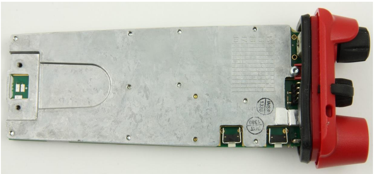
Transceiver module 3965 (PCB top): 60-150001
