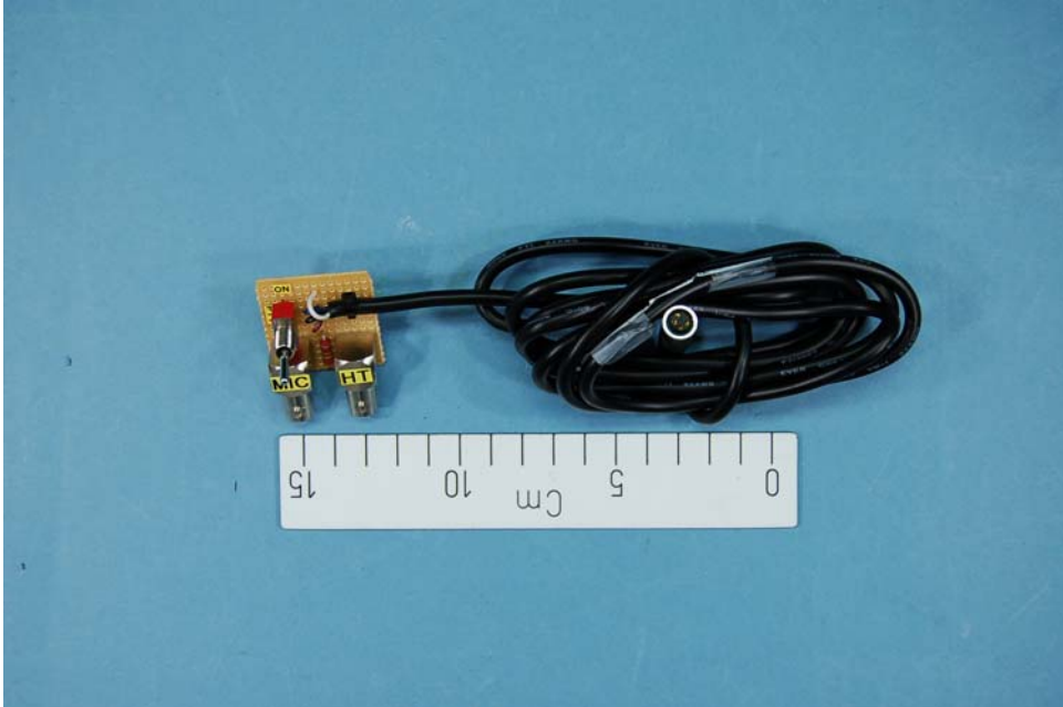
Test jig for microphone & Loudspeaker
