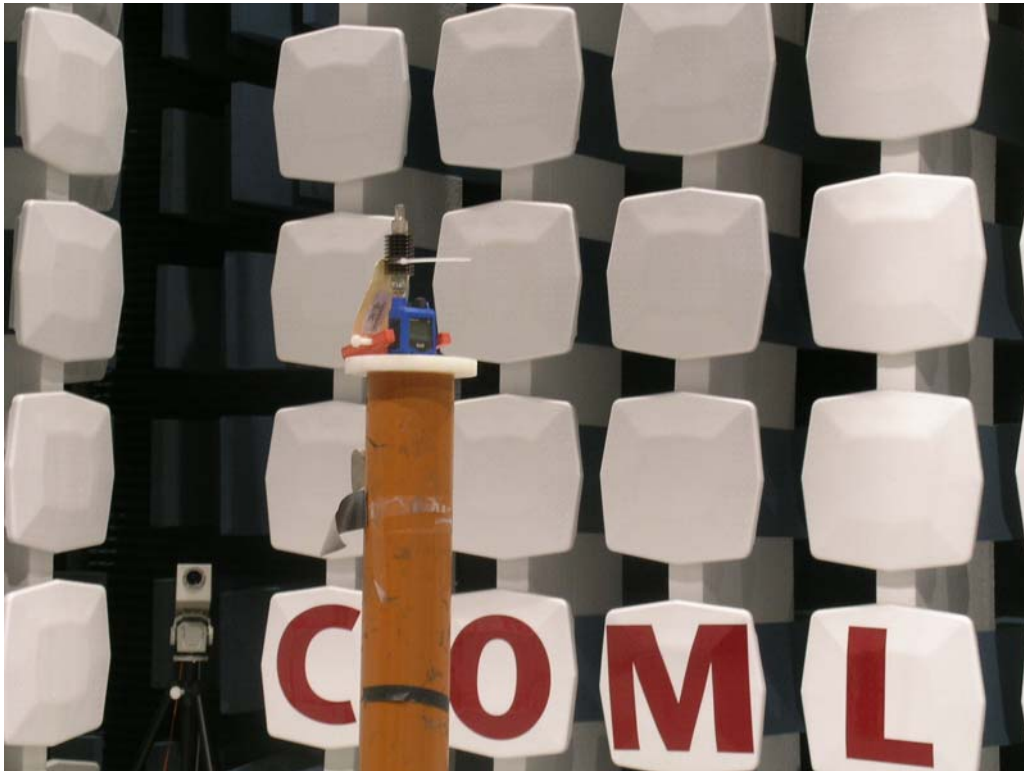
Test set-up for radiated measurements – 50 ohm load
