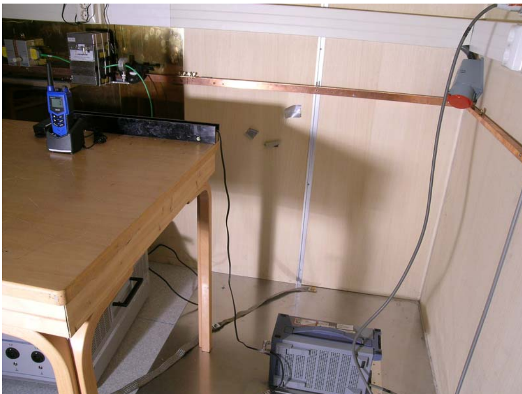
115Vac , 60Hz – Power line conducted emission
