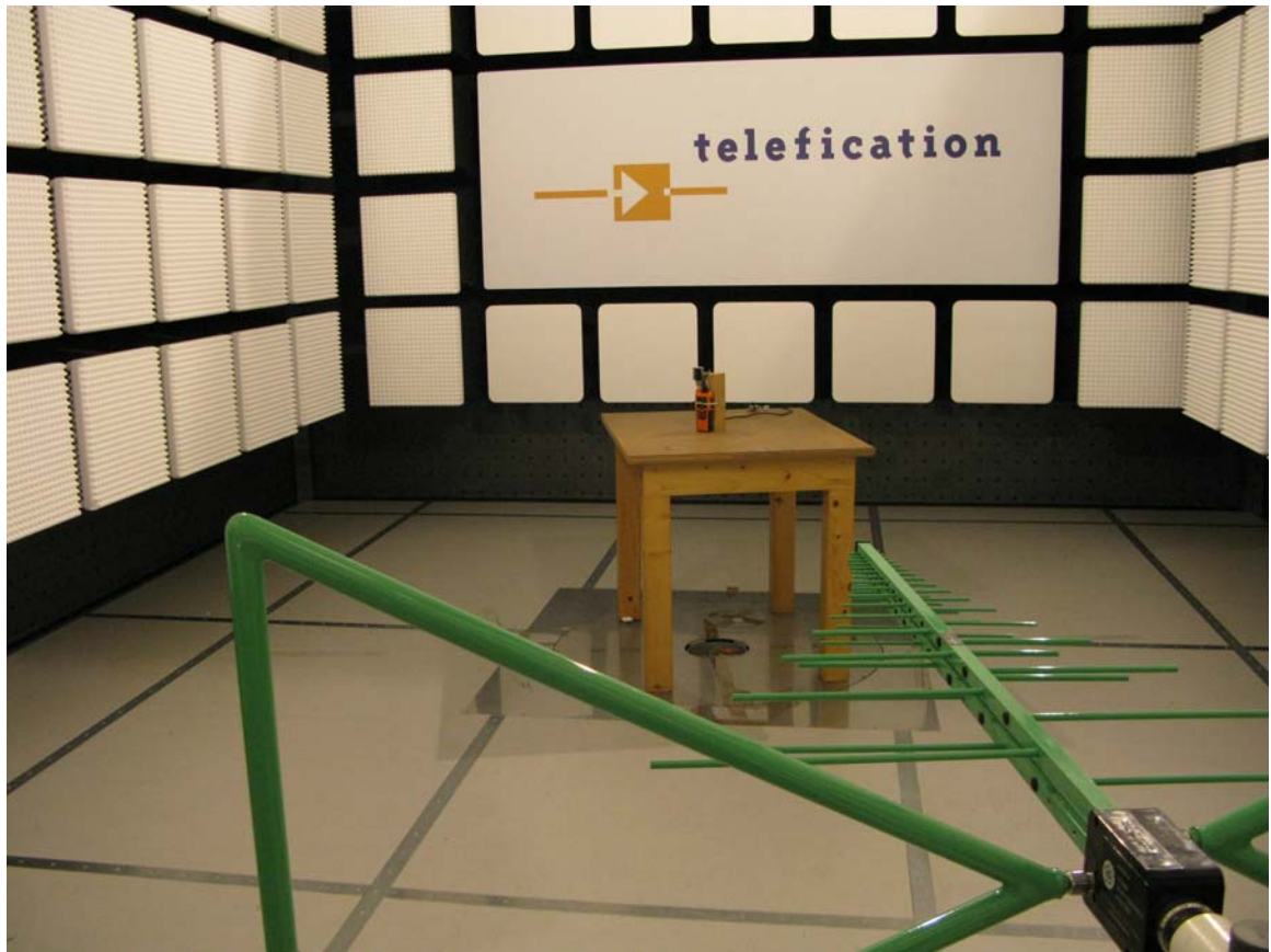
Photograph 1: Test setup cabinet radiation (> 30 MHz)
