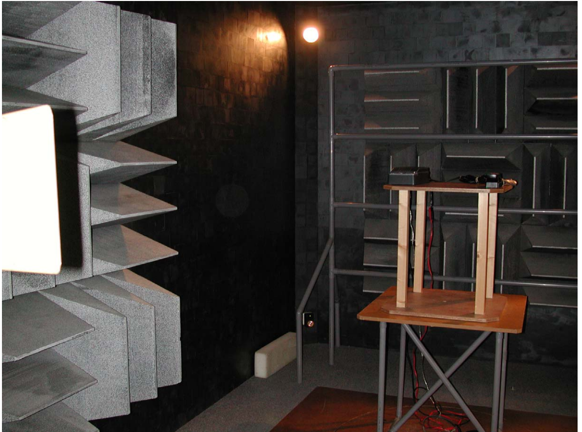
Photograph 3: Radiated emissions (1 – 18 GHz) test set up.
