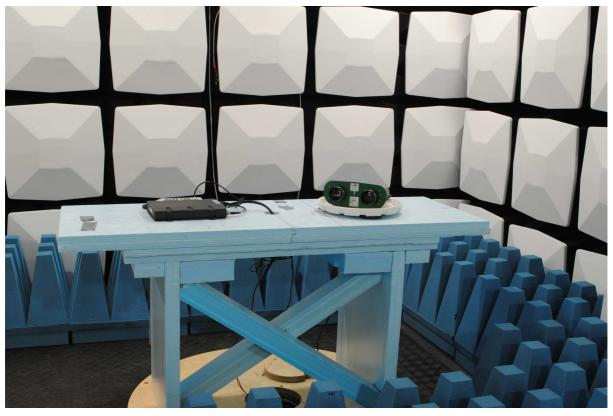
Test setup for radiated emissions:
