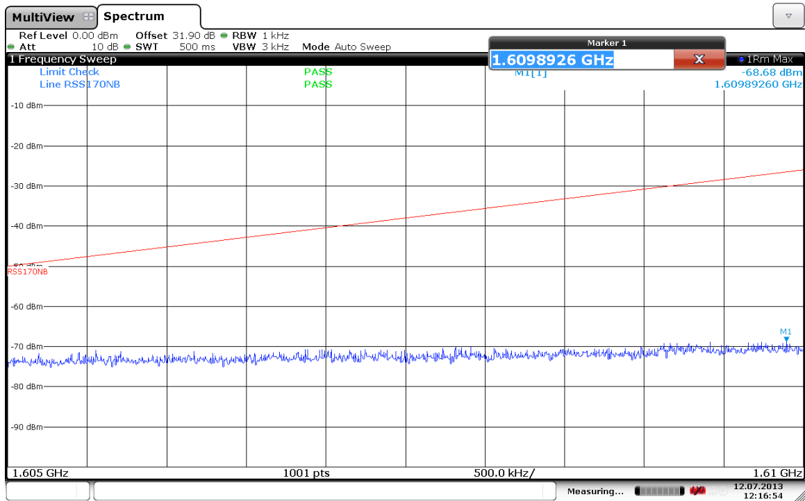
Additional Unwanted NB Emissions, fr80t5x4, 1626.6 MHz
