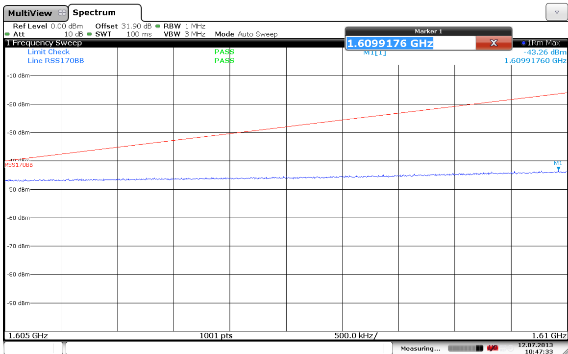
Additional Unwanted BB Emissions, fr80t5x4, 1626.6 MHz
