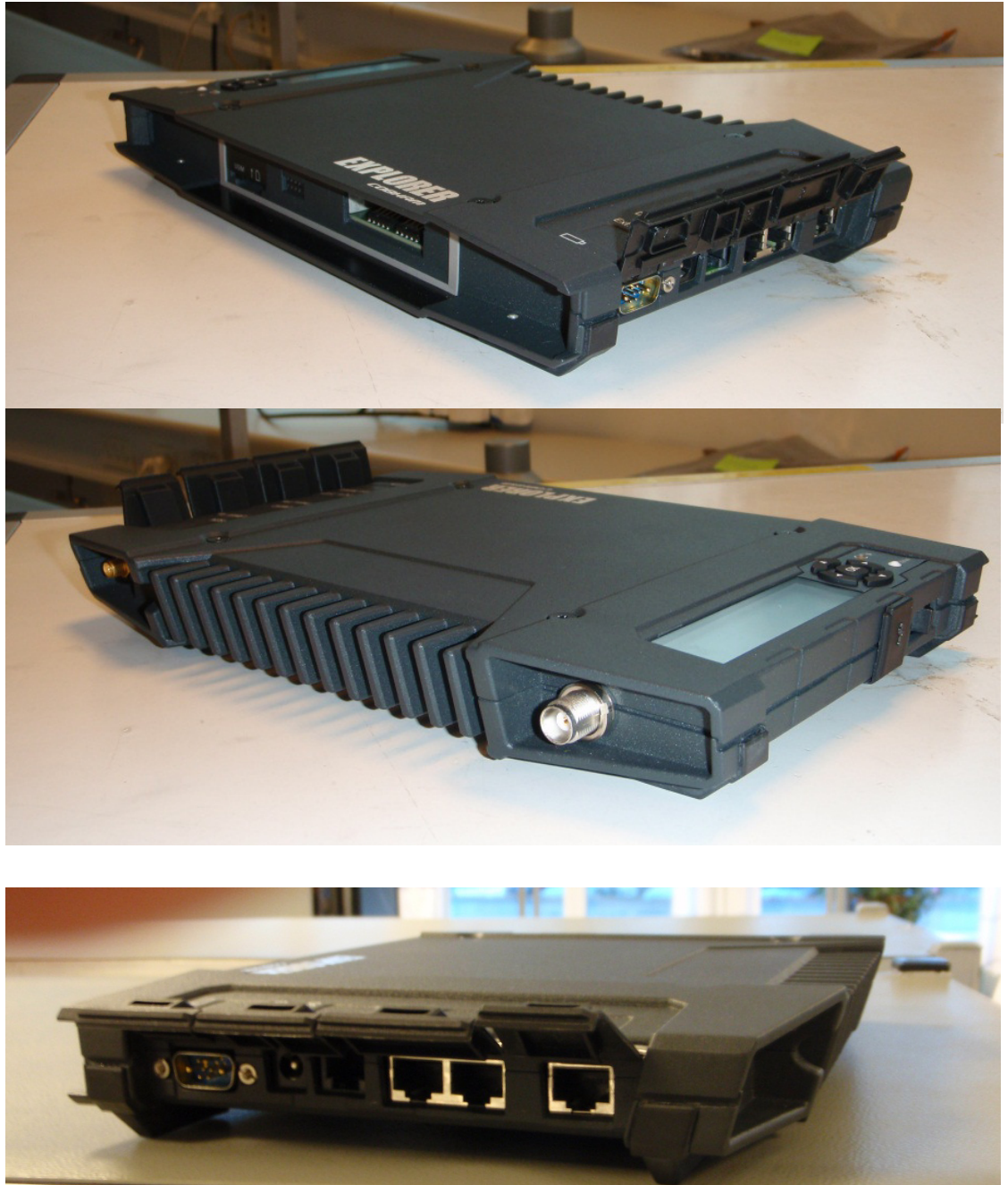
Figure 4 Connectors on Explore 710 Transceiver unit TT-3732B
