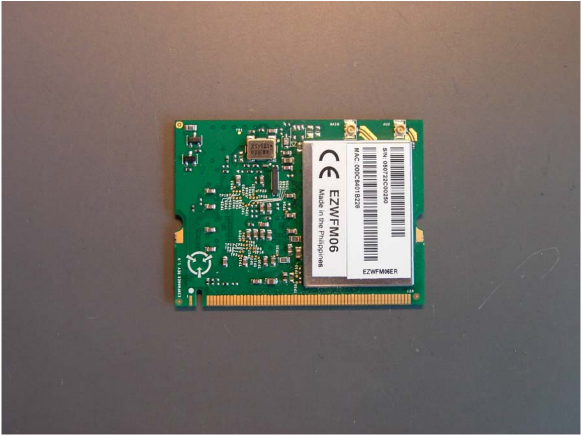
Figure 9 WLAN card with shield
