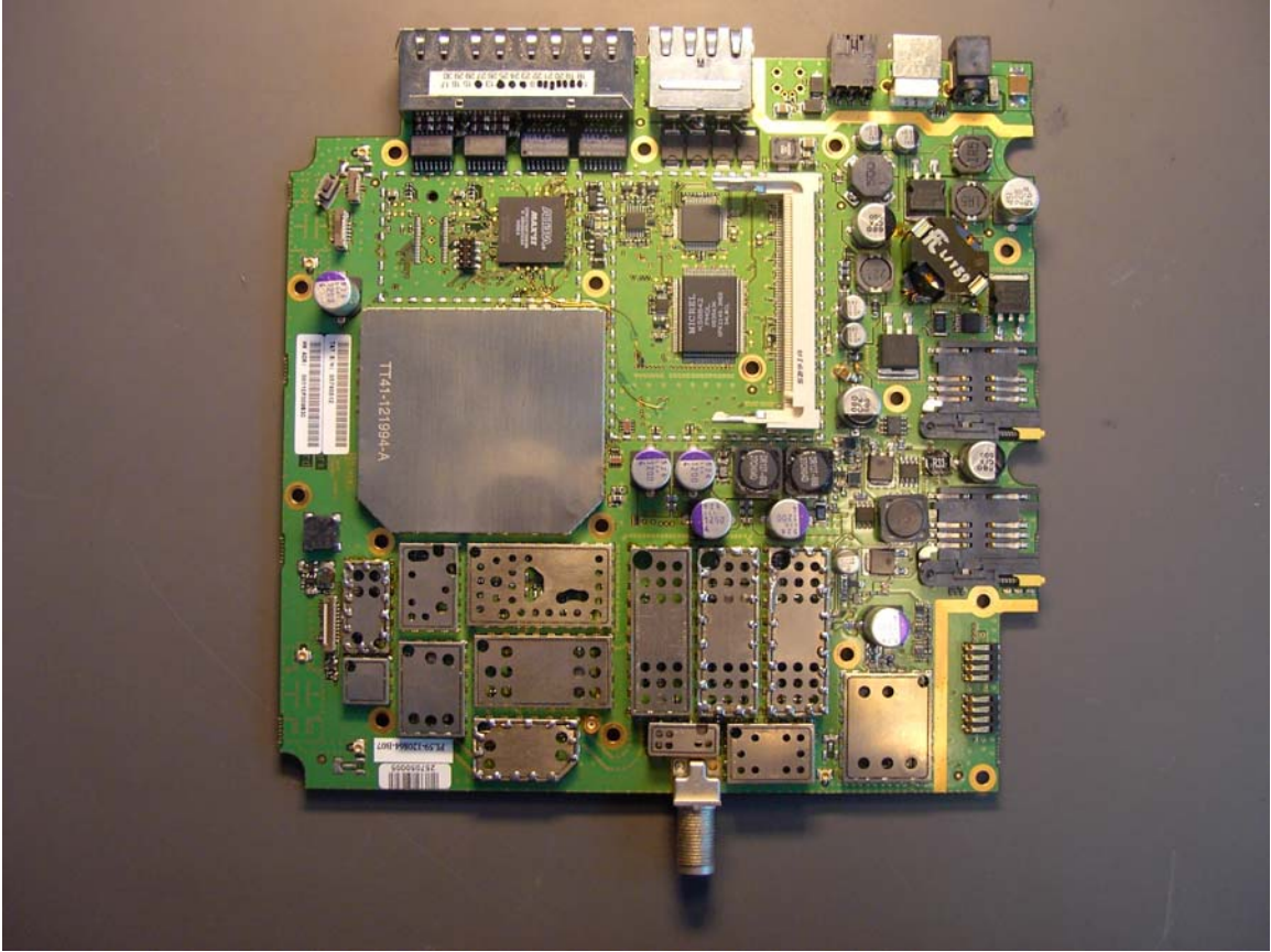
Figure 5 Transceiver Module with shields
