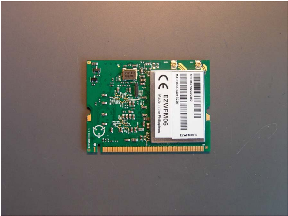
Figure 9 WLAN card with shield
