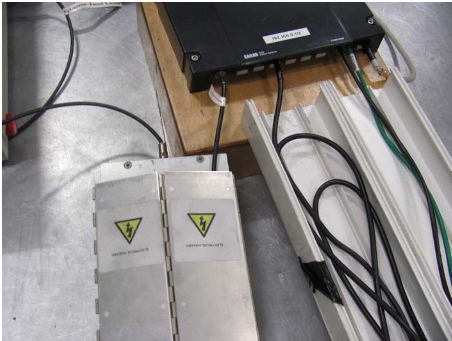
Immunity to Fast Transient Bursts Common Mode (Signal, Control and Telecommunications Port)
