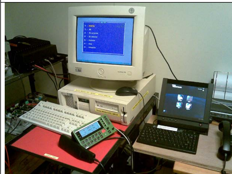
RES-TEST SYSTEM of verification of the software and algorithms of functioning NBDP GMDSS equipment
