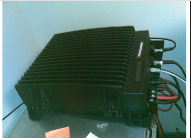
SAILOR 6363 250W MF/HF Class A Transceiver Unit
