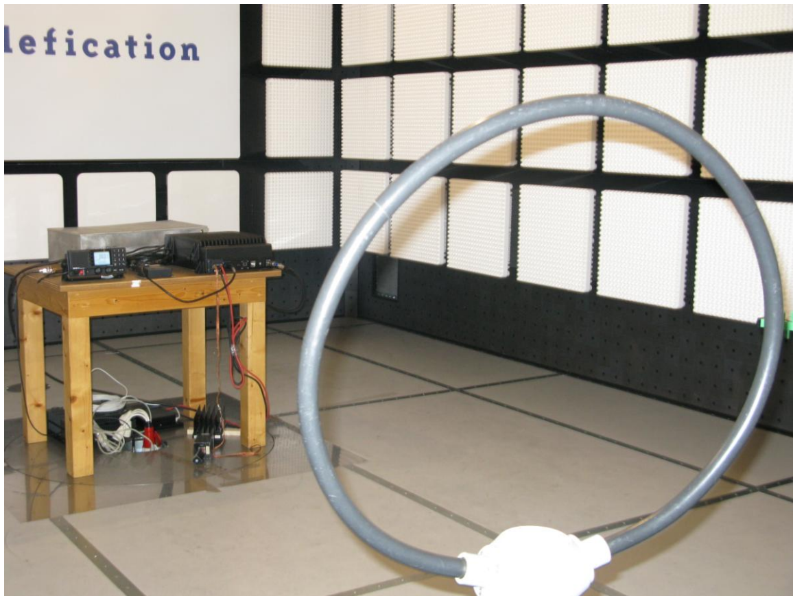
Photograph 1: Test set up radiated emissions up to 30 MHz
