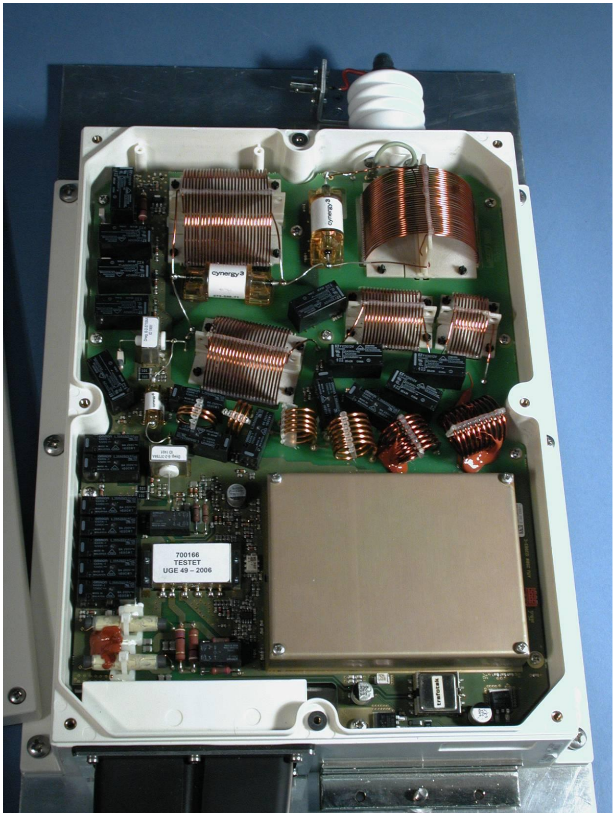
Photograph 6: Antenna tuning unit. inside view
