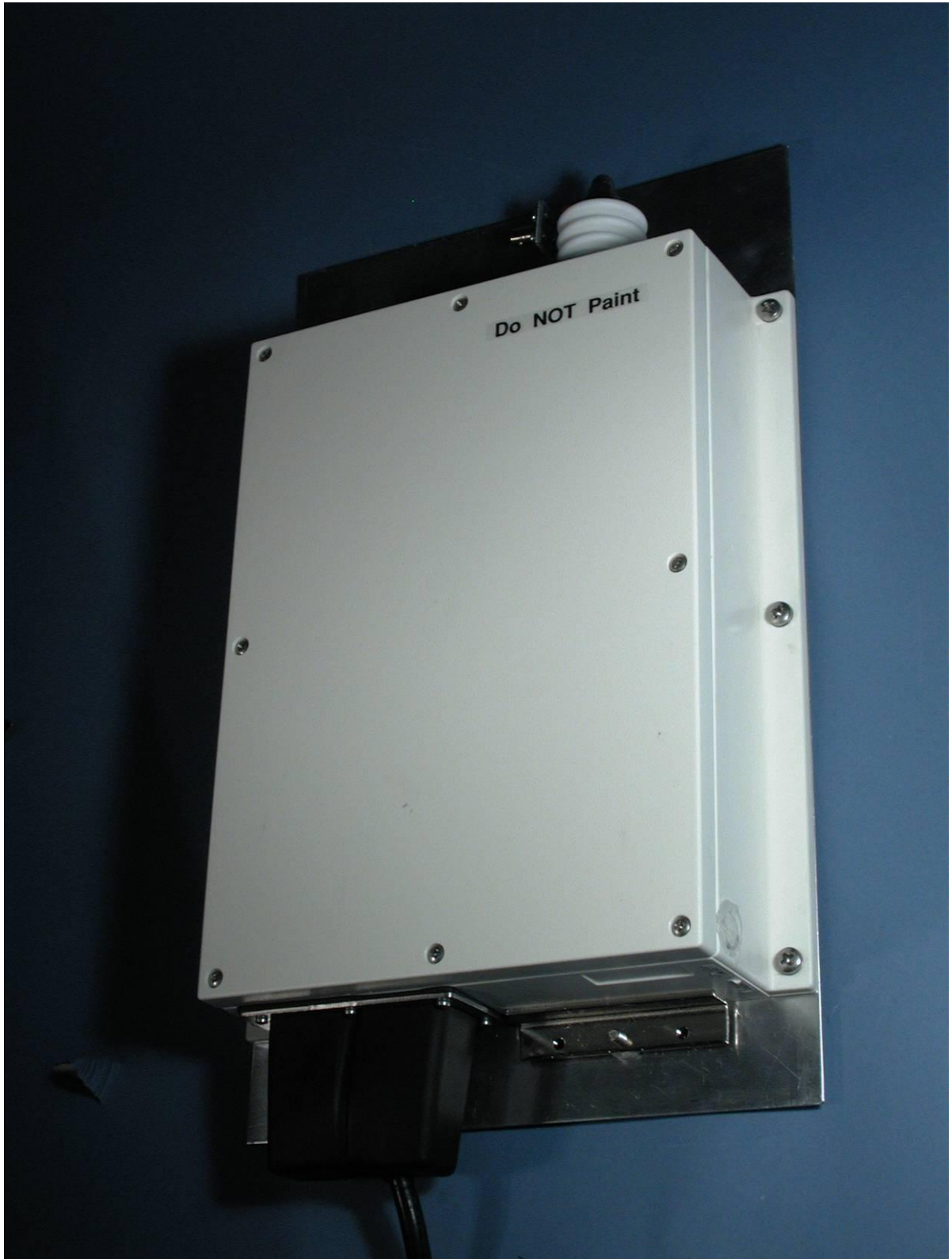
Photograph 7: Antenna tuning unit
