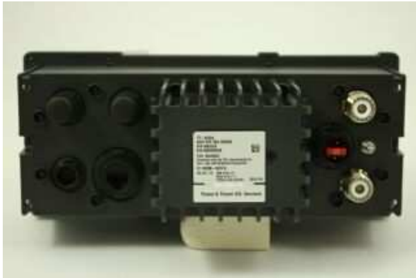
Placing of type label for 6222 VHF at back side
