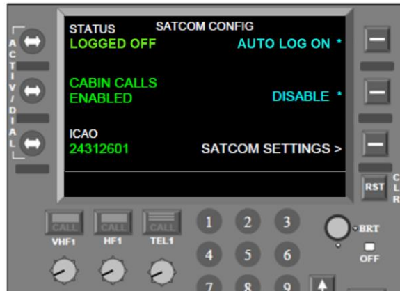
Figure 5-16: RMP - SATCOM Config - Status - Logged Off
