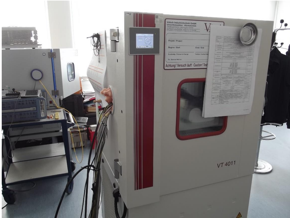
Photo 12: EUT inside climatic box
