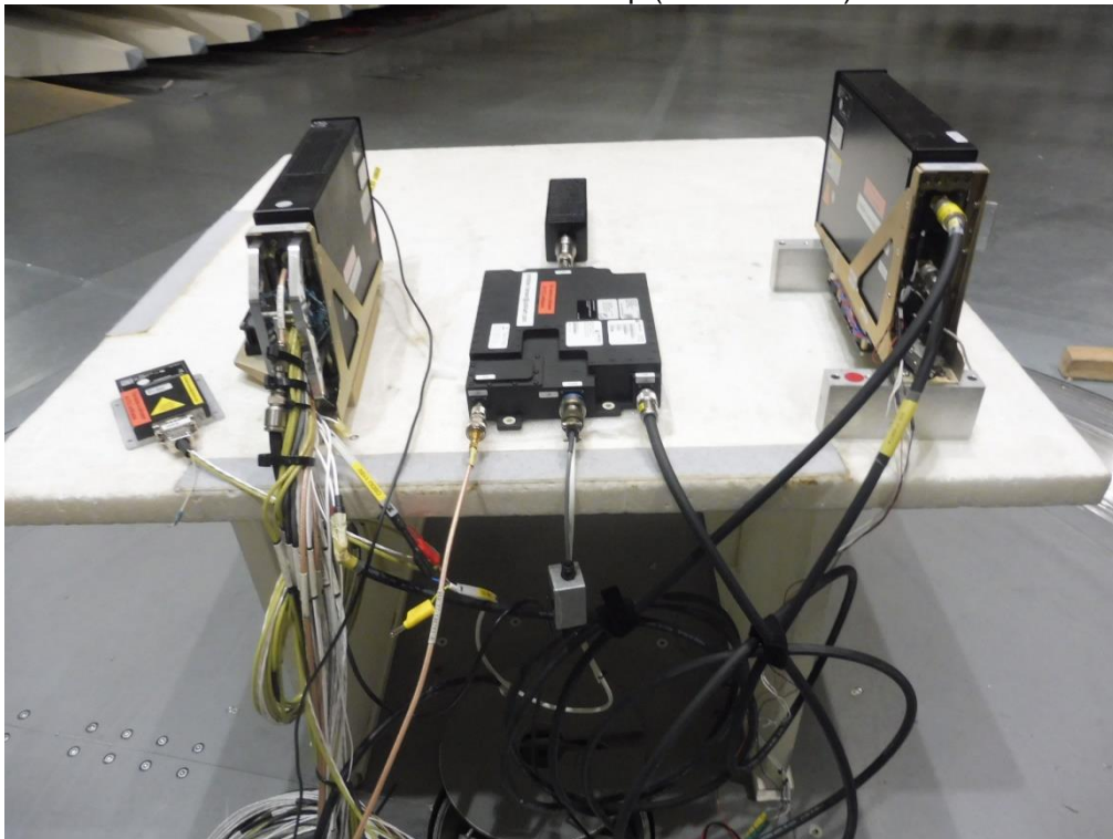
Photo 4: radiated test set-up (10m chamber)
