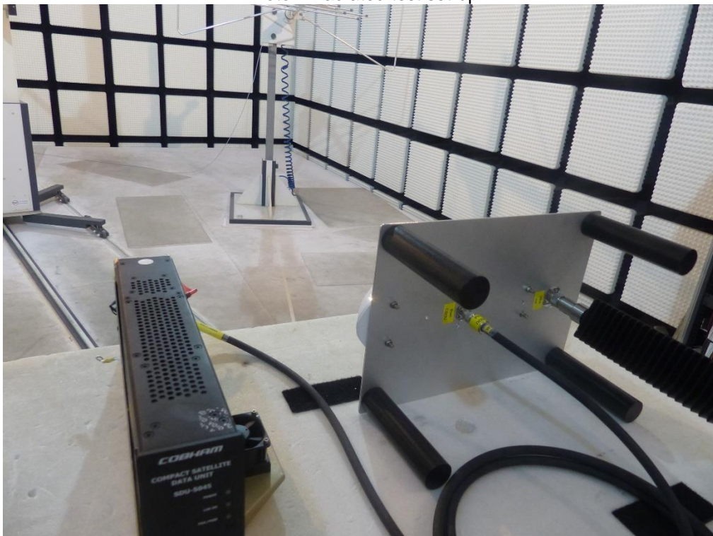
Photo 2: radiated test set-up
