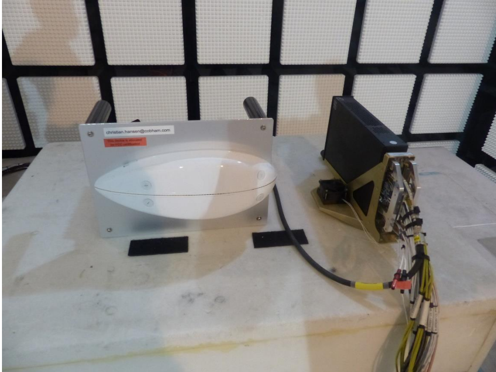
Photo 1: radiated test set-up
