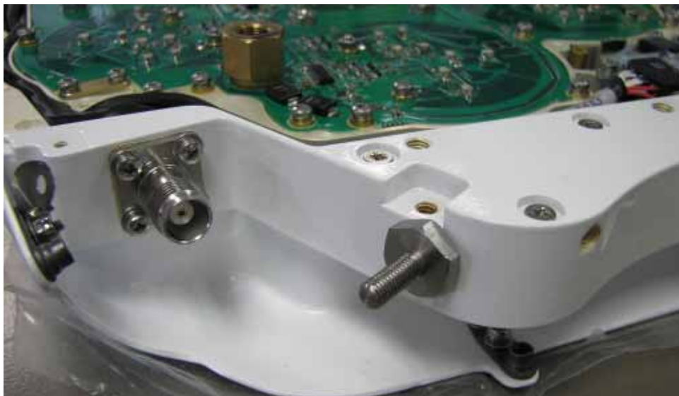
Figure 8: The additional grounding stud on the HGA-7001
