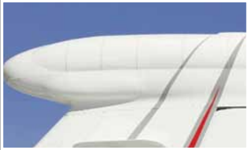
The AMT-700 is typically housed under a tail-mounted radome, but can also be mounted at several locations on the fuselage.
