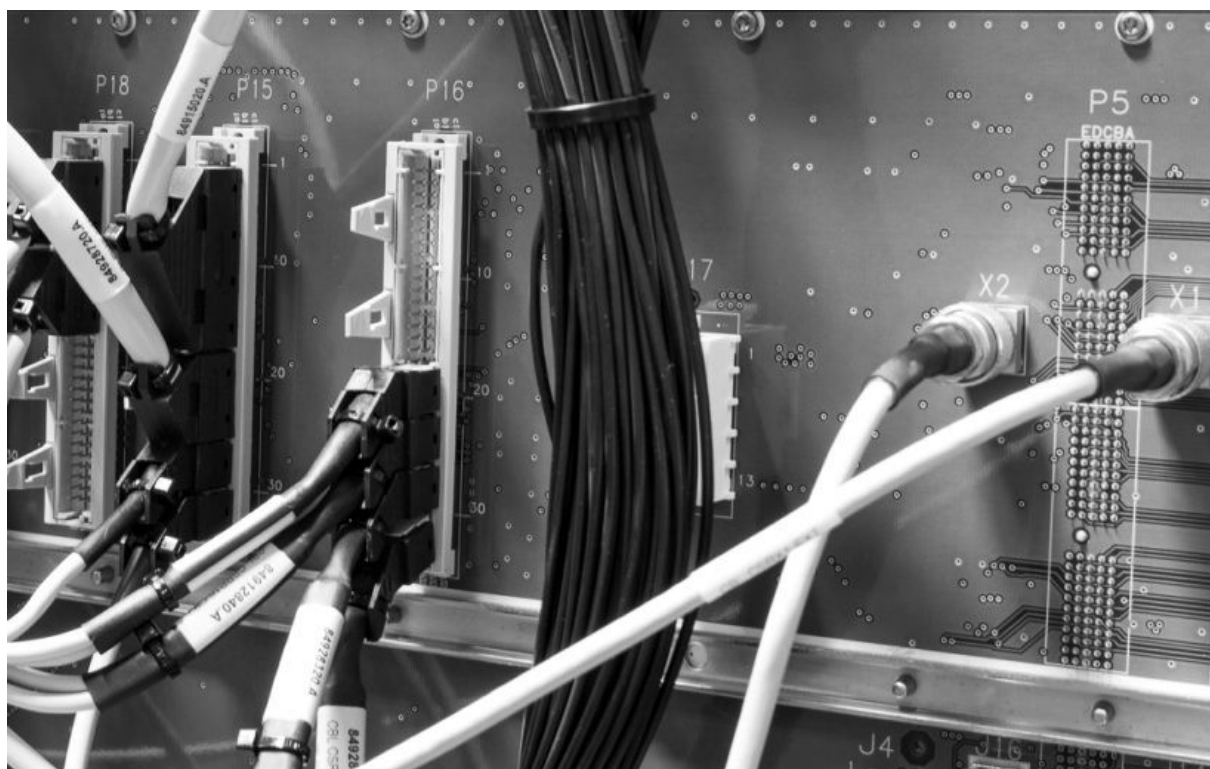
Figure 66 : Basic cabinet, common subrack, connectors for P15, P16, P18 and X1, X2
