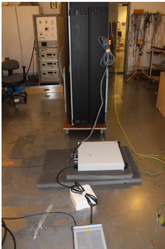
Photograph 2. Conducted emissions at the mains ports.
