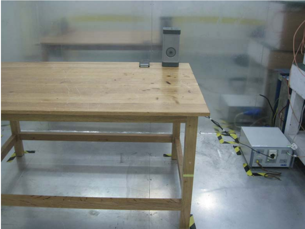
Radiated Measurement Photos (Below 1GHz)
