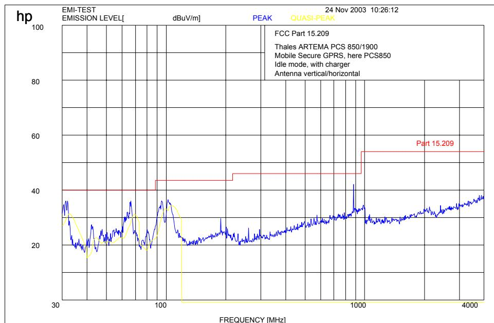
**Idle mode up to 12 GHz (850 MHz with Charger)**
