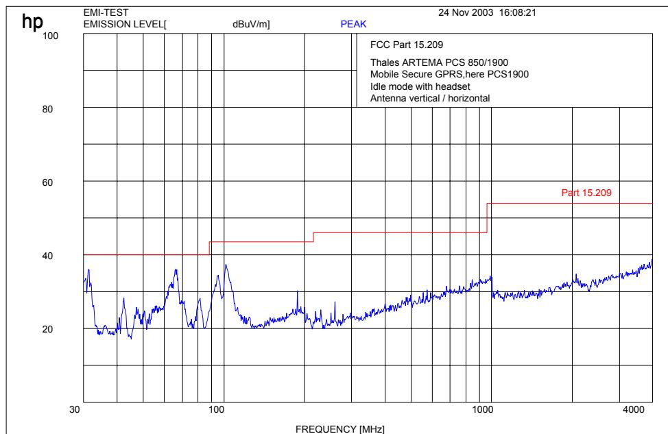
**Idle mode up to 12 GHz (1900 MHz with Headset)**
