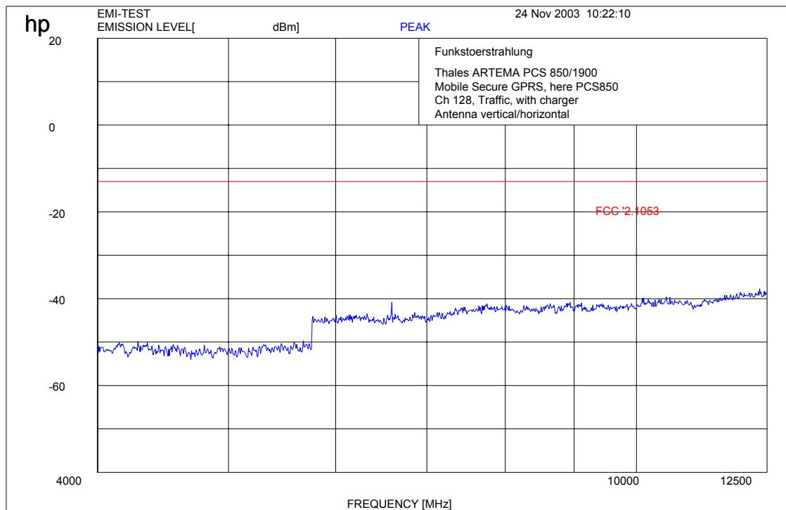
**$f < 1 \text{ GHz}$  : RBW/VBW: 100 kHz** **$f \geq 1 \text{ GHz}$  : RBW/VBW 1 MHz****Carrier suppressed with a rejection filter****REFERENCE NUMBER(S) OF TEST EQUIPMENT USED****(for reference numbers see test equipment listing)**
