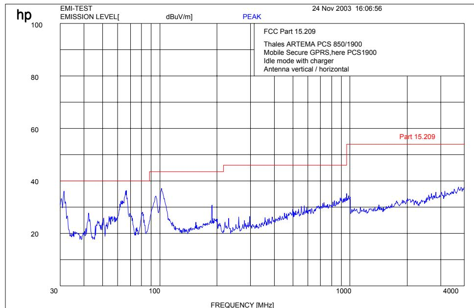
**Idle mode up to 12 GHz (1900 MHz with Charger)**
