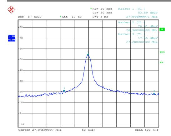
Eastern times wireless mouse model DS-2131 Out of band emiss ion Date: 29.MAR.2006 10:19:42
