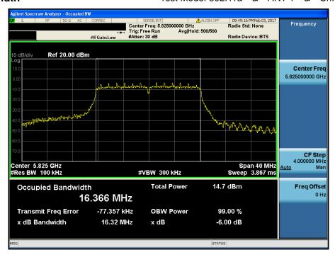
6 dB Bandwidth Test Mode: 802.11n HT20 & ANT 1 & Ch.149
