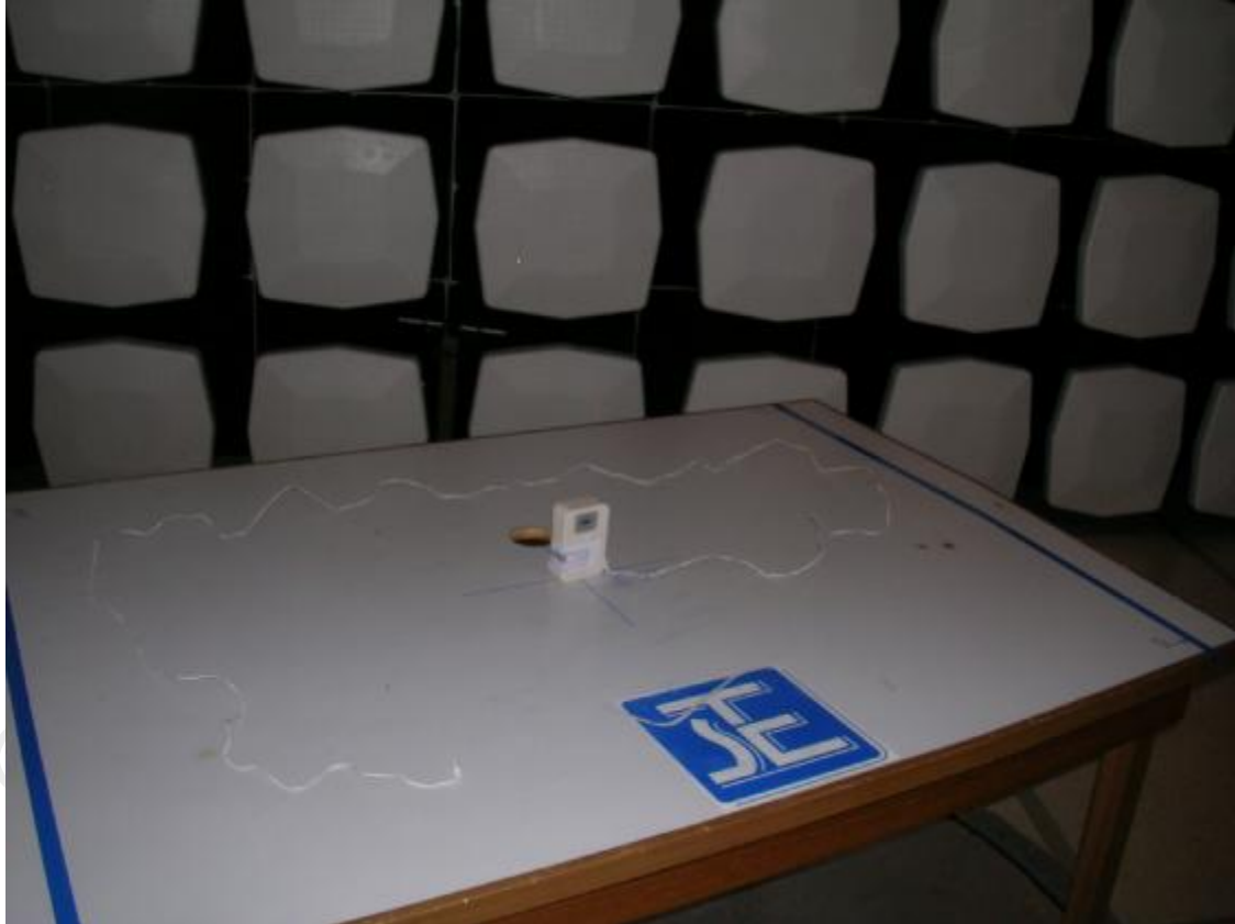
Measurement of Radiated Emission Test Set Up
