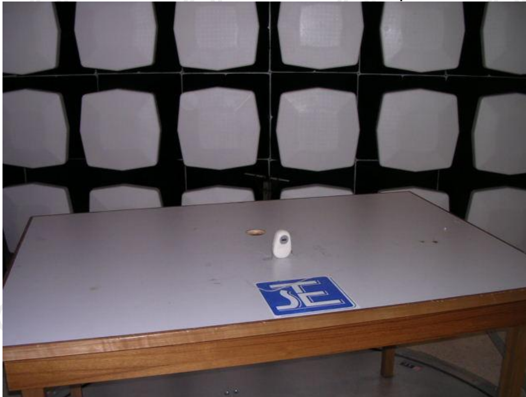
Measurement of Radiated Emission Test Set Up
