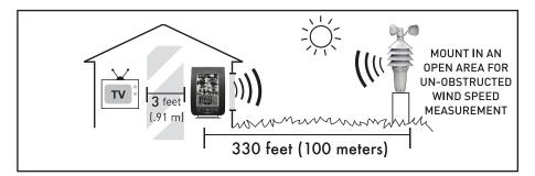
Now that setup is complete and you understand how to operate the weather station, you must choose a location to place the wireless sensor and the main unit. The wireless sensor MUST be placed less than 330 feet (100 meters) away from the main unit.
